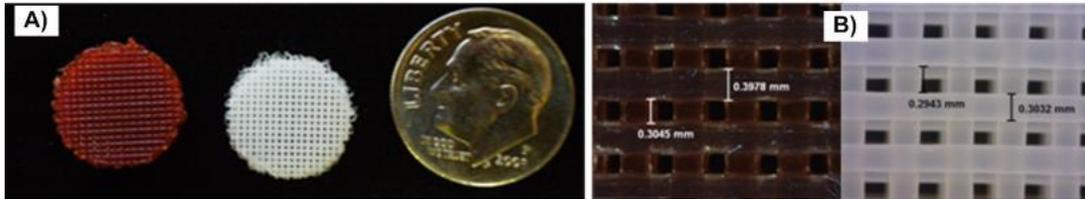
**Figure 6.** (a) Printed ICW (red) and ABS (white) scaffolds patterns with (b) a gap width of 0.30 mm.
