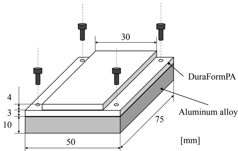
Figure 2 Base plate structure
