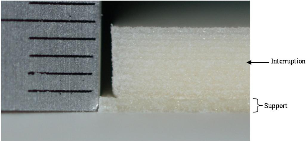
**Figure 11** Closed-up side view of a part whose process was interrupted for 30min. Suspended layer is indexed by the arrow.
