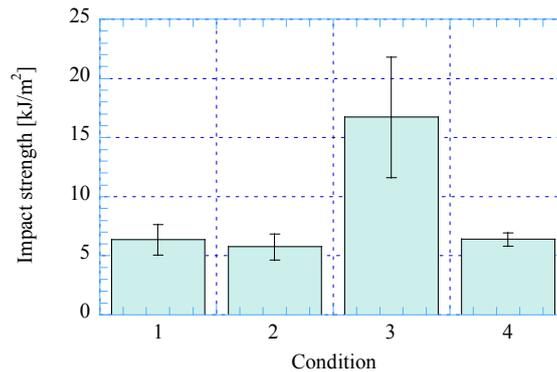
**Figure 10** Impact strengths in various conditions. Izod unnotched (ISO 180)
