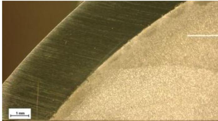
**Fig. 8:** Cross section of shaft cladding
