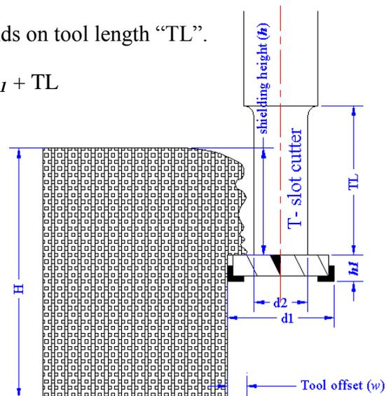
Figure (6): Tool dimensions condition of the process
