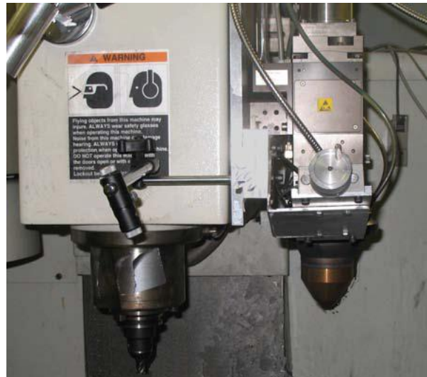
Figure (3): Integrated 5-axis FADAL CNC and Laser Deposition Head
