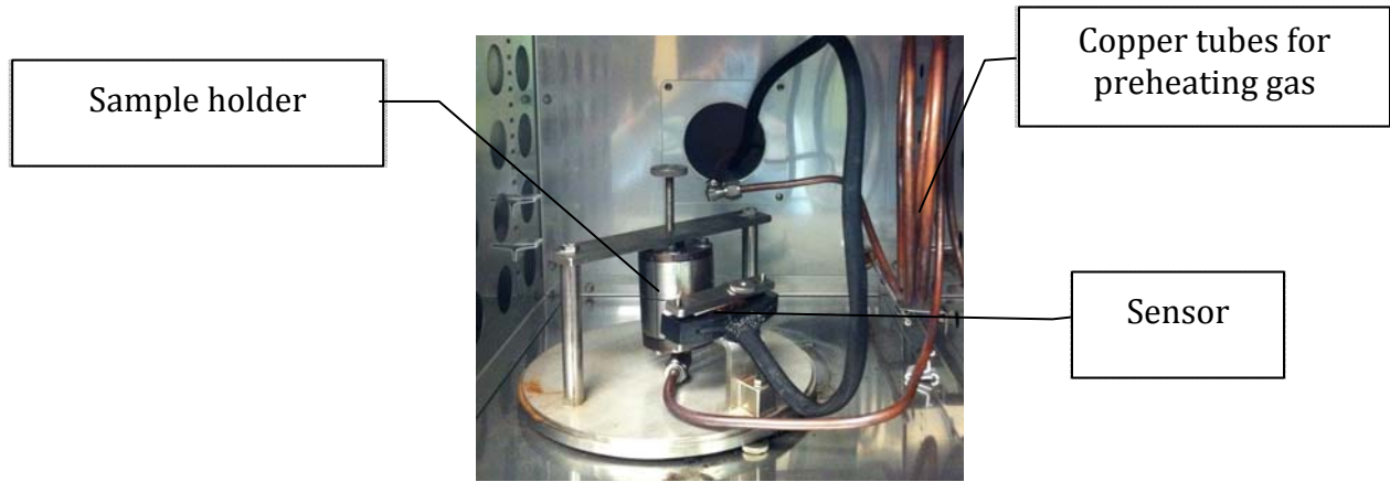
Figure 1: Experimental apparatus for measuring the thermal conductivity of polyamide-12 powder. The view is inside the temperature control oven, which includes the sample holder, rack, copper tubes and sensor.
