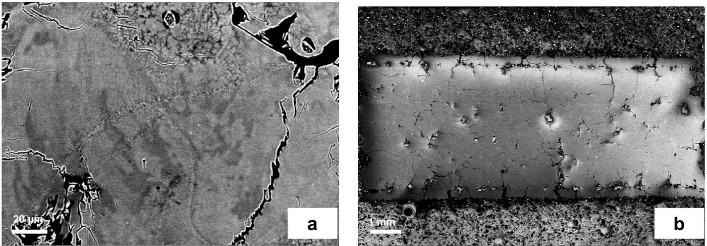
Figure 3: a Detailed SEM BSE picture of the SLM produced cylinder and b SEM overview of a whole cylinder cut in half
