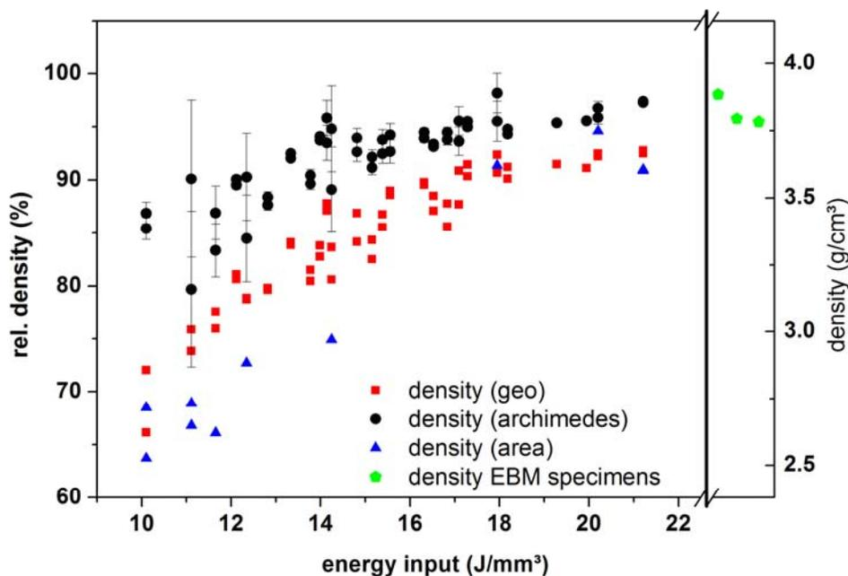
Figure 4. Relative and absolute density in dependence of the energy input of the produced SLM parts via geometric, Archimedes and area method and relative and absolute density of the EBM specimens before hipping
