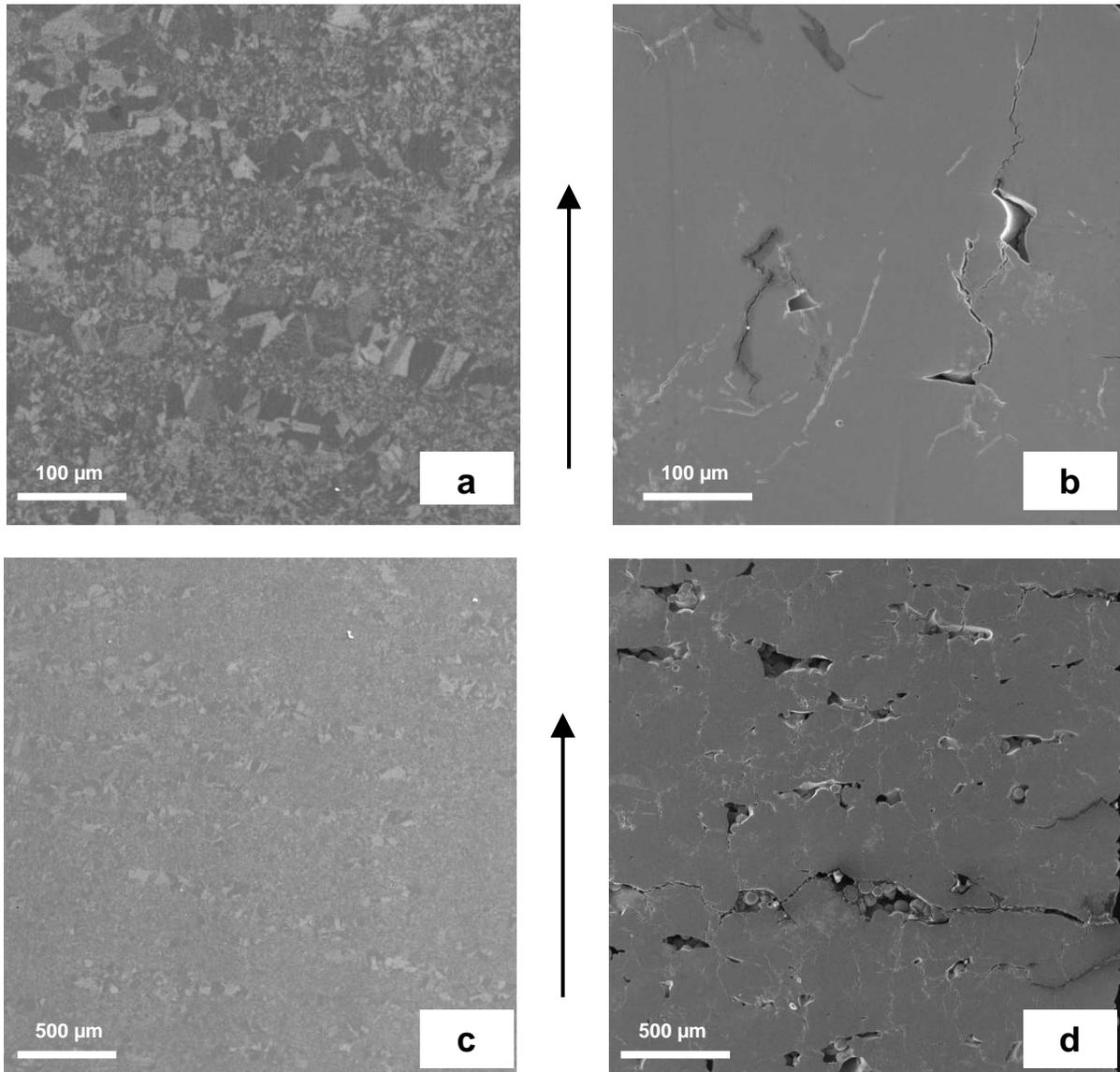
Figure 6: SEM picture of the microstructure of one of the a) EBM produced and b) SLM produced cylinders and more detailed picture of the same c) EBM specimen and d) SLM specimen (the arrow indicates the building direction)
