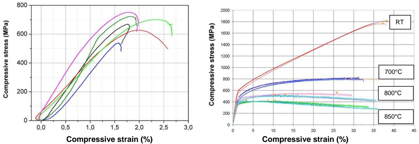
Figure 8 Results of the compression test a at room temperature of the as produced SLM specimens and b of the as produced EBM specimens at room temperature and at 700, 800 and 850°C
