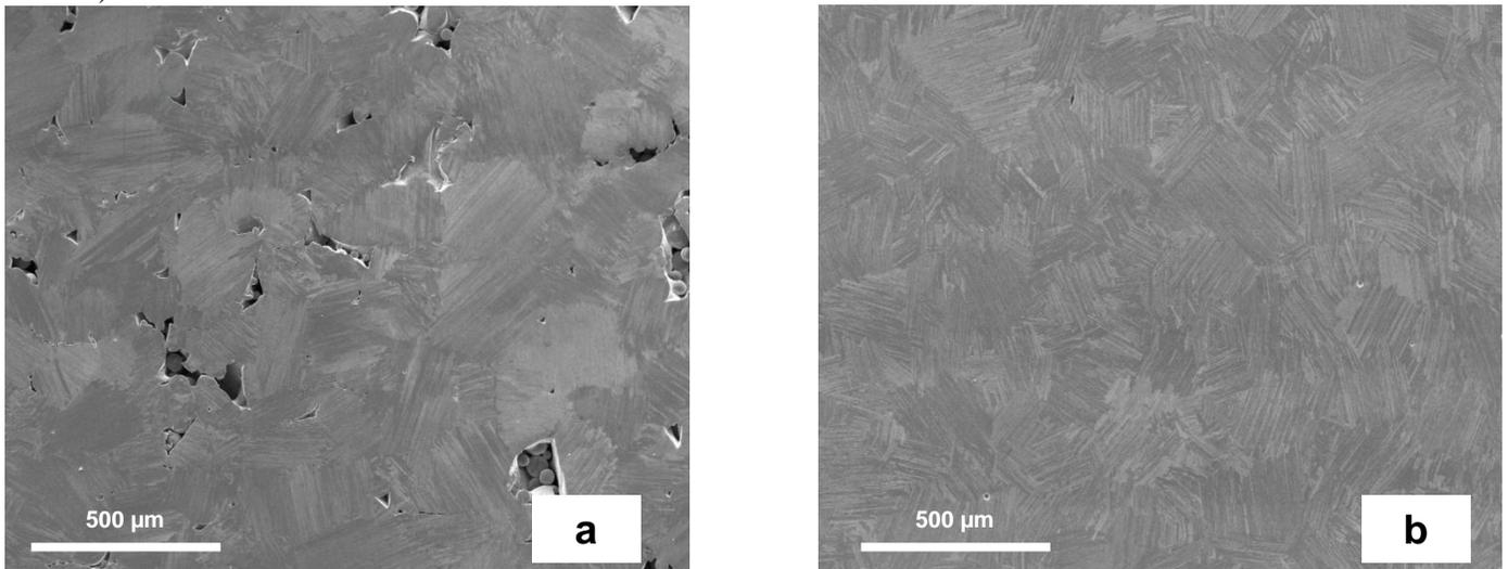
Figure 7: SEM picture of the microstructure of one of the a) EBM produced and b) SLM produced cylinders after heat treatment
