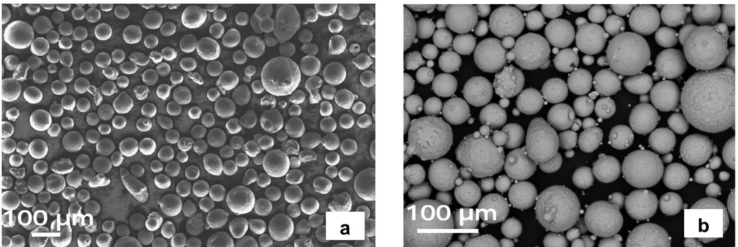
Figure 2. a SEM picture of the used powder for EBM and b SEM picture of the used powder for SLM
