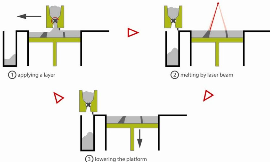
Figure 1 Three step iterative process of additive manufacturing
