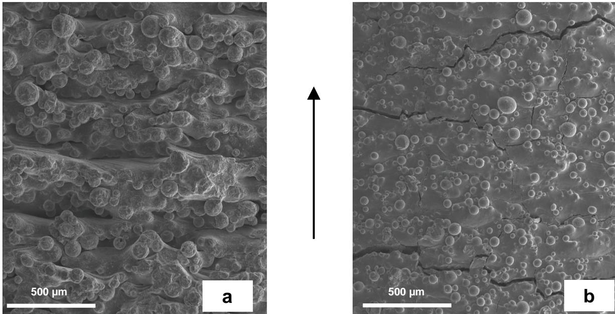
Figure 5: SEM picture of the surface of the specimens a) EBM, b) SLM (the arrow indicates the building direction)
