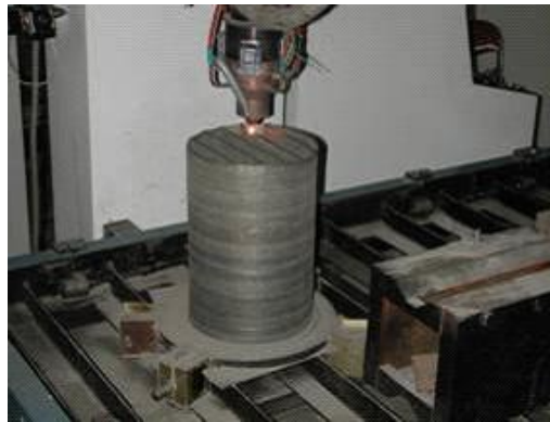
Fig. 10 AM process based on high-energy laser beams
