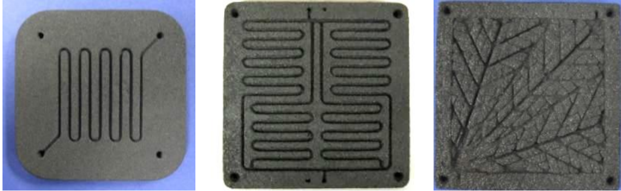
Figure 4. Example bipolar plates fabricated by the SLS process
