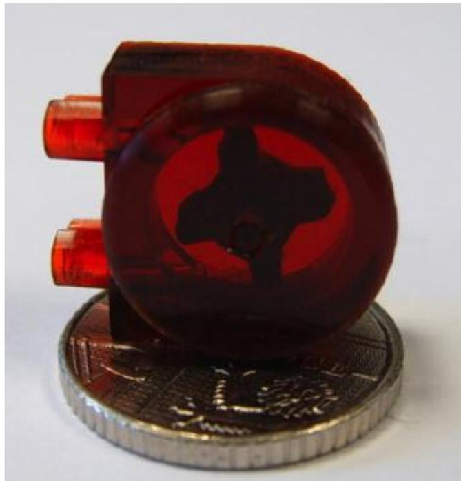
**Figure 10: Flow sensor device fabricated using MSL [24]**
