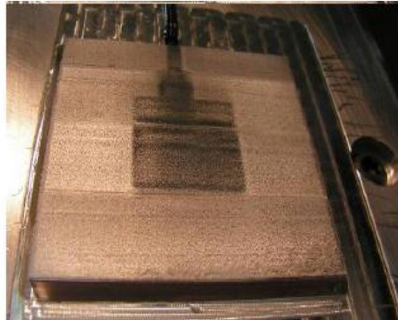
**Figure 6: Ultrasonic consolidation of aluminum onto embedded sensor [19]**
