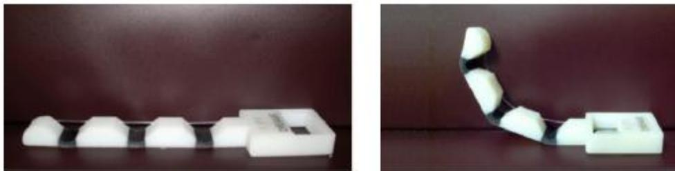
**Figure 7: Actuated finger created using Objet PolyJet 3D Printing Machine [20]**
