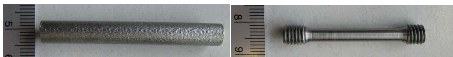
Figure 1: Tensile specimens (190W, 800mm/s) – horizontally produced blank (left) and final drilled specimen according to DIN-50125-form B (right).
