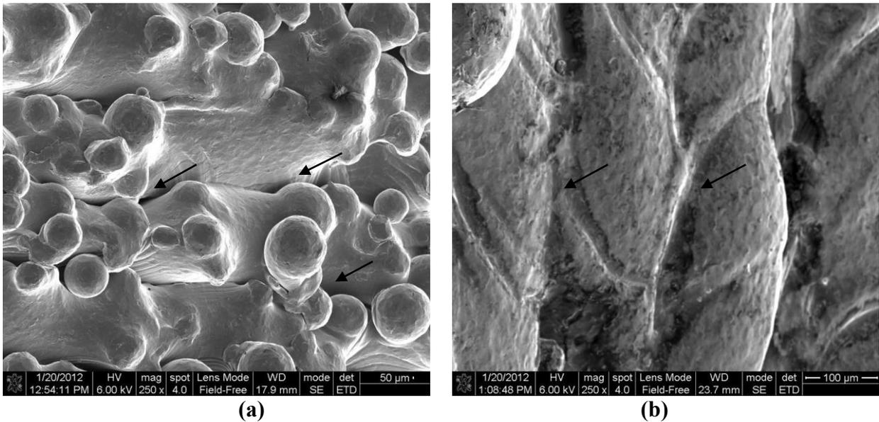
Fig.4. SEM images of the external surfaces of EBM built samples a) Vertical built sample b) Horizontal built sample (arrow indicates ridges/valleys at the surface)
