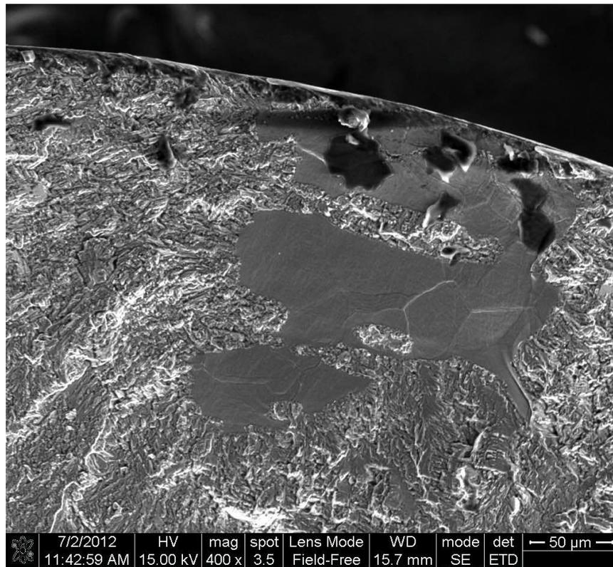
Fig.6. SEM image showing brittle mode of crack initiation for a machined part
