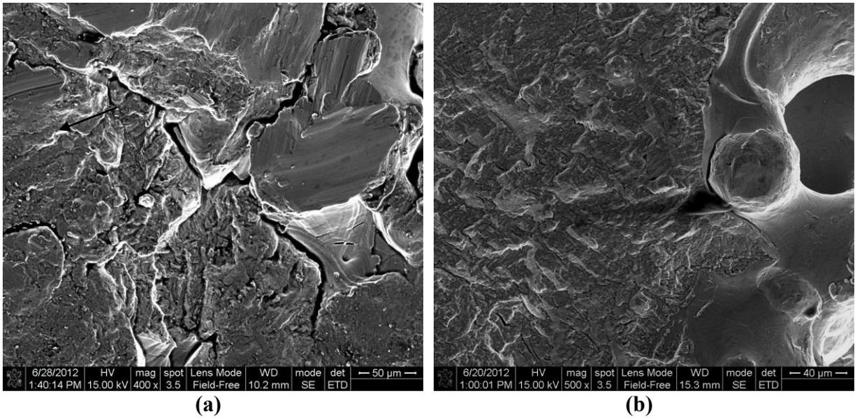
Fig.5. SEM image showing fatigue fracture surfaces (crack initiation points): a) vertical as-built b) horizontal as-built
