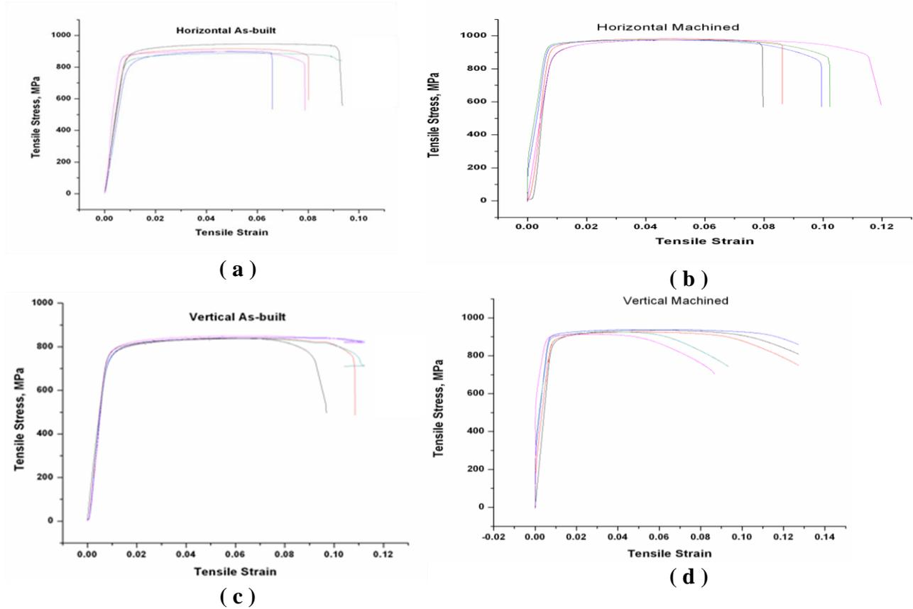
Fig.1. Stress-Strain curves for EBM built Ti64 samples. a) Horizontal as-built b) Horizontal machined c) Vertical as-built d) Vertical machined
