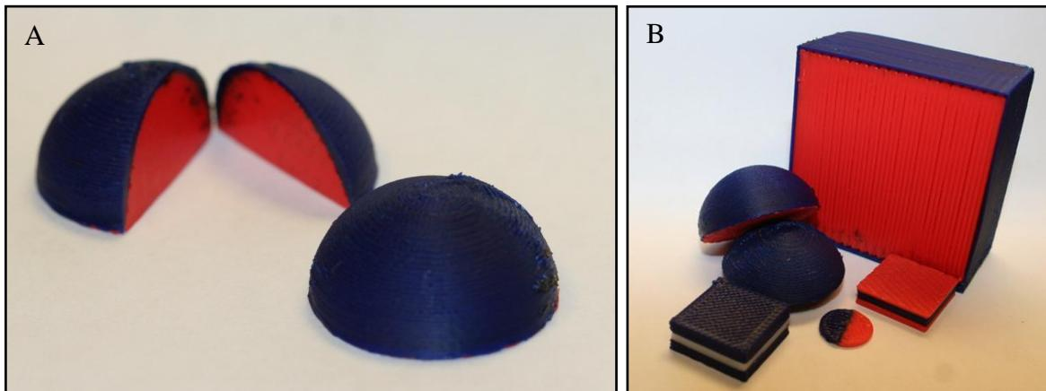
**Figure 7:** ABS parts demonstrating the variable layer thickness and road width approach. A) dome structures (structure in background was bisected after being fabricated). B) additional parts demonstrating the use of different colored polymers to achieve aesthetic requirements.
