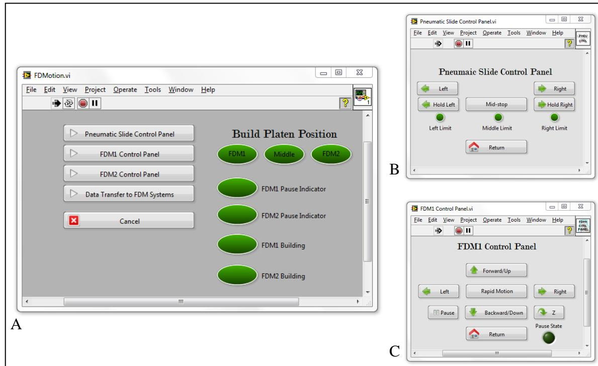
**Figure 4: Graphic user interface for FDMotion software. A) main control panel for FDMotion. B) control panel for pneumatic slide. C) control panel for FDM1 system.**
