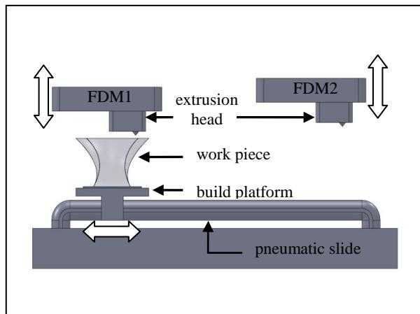
Figure 2: Schematic of multi-material, multi-technology FDM system
