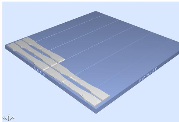
**Figure 5.** Build platform layout for “YXT” (specimens oriented in the y-axis, flat z-orientation, and tight part spacing) experiment.
