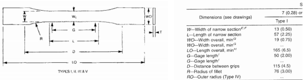
**Figure 6.** ASTM D638 Type 1 specimen dimensions
