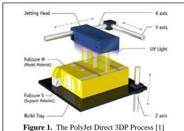
For example, by simultaneously jetting "TangoBlack" (an elastomeric material) and "VeroWhite" (a rigid polymer), a designer is able to manufacture products with functionally graded material properties. As such, PJD-3DP offers design freedom in specifying both the placement and the properties of materials on a point-by-point basis.
