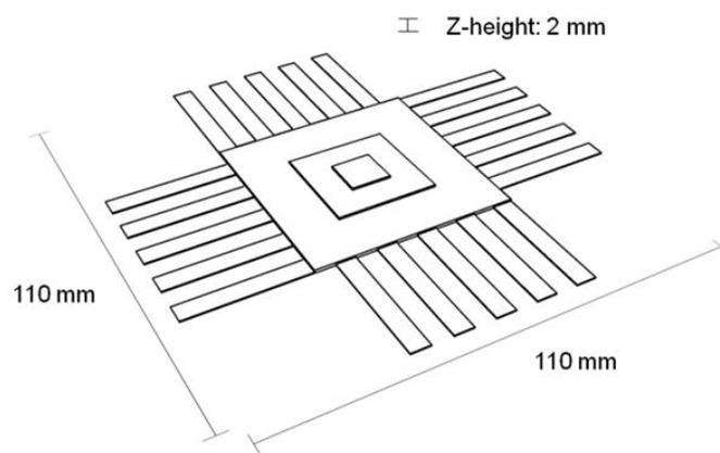
**Figure 3: Design of the power monitoring test part**
