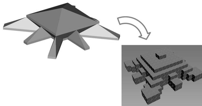
**Figure 1: Conversion of a test part into a voxel approximation**
