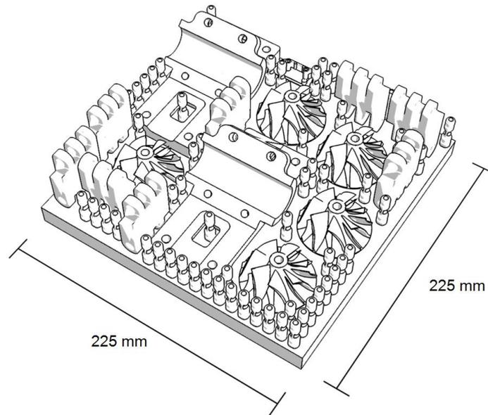
**Figure 4: Full build configuration of basket parts**
