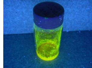
Figure 2: QD Powder in UV Light (Yellow Color)
