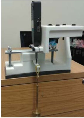
Figure 4 Positioning of the specimen during bending
