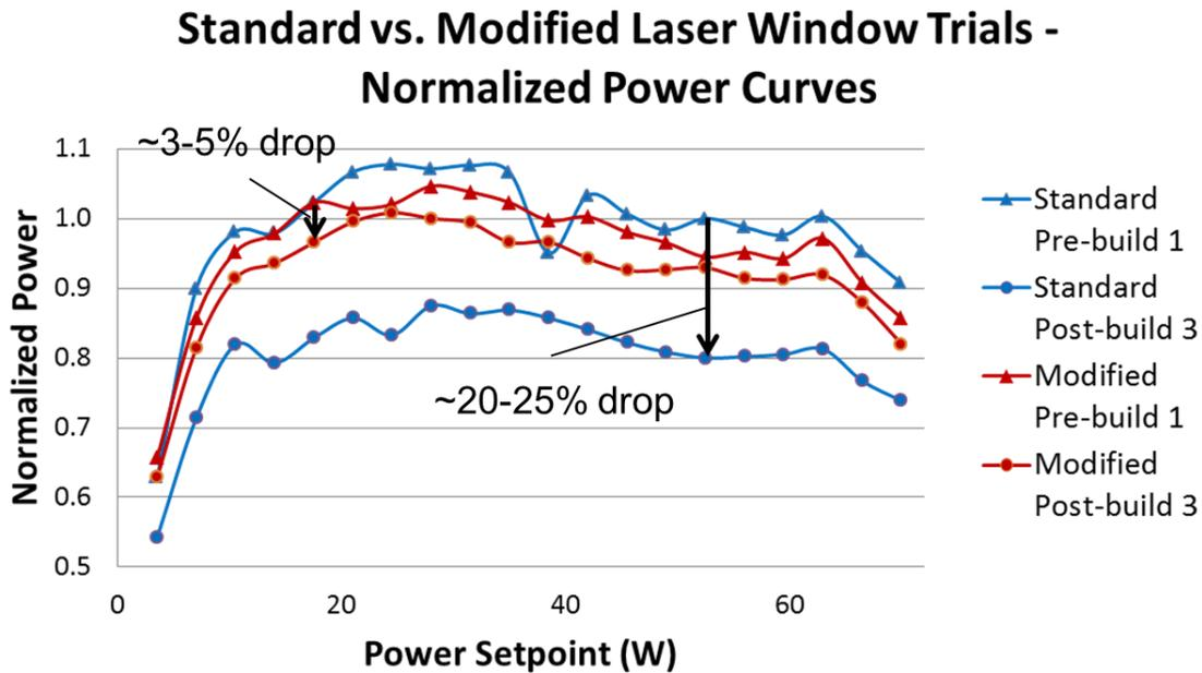
**Figure 11.** Standard design and modified design power curves overlaid
