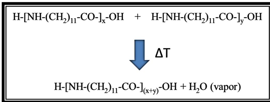
**Figure 2.** *Post-condensation reaction for PA 12*
