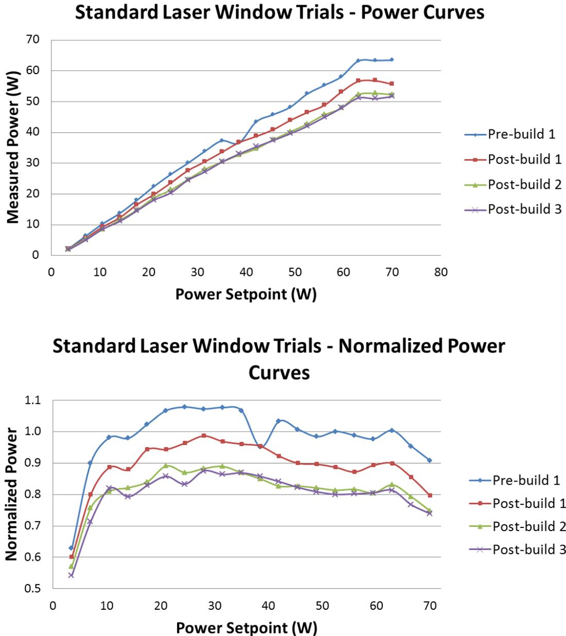
**Figure 3.** *Nominal and normalized power curves for the standard window housing design*
