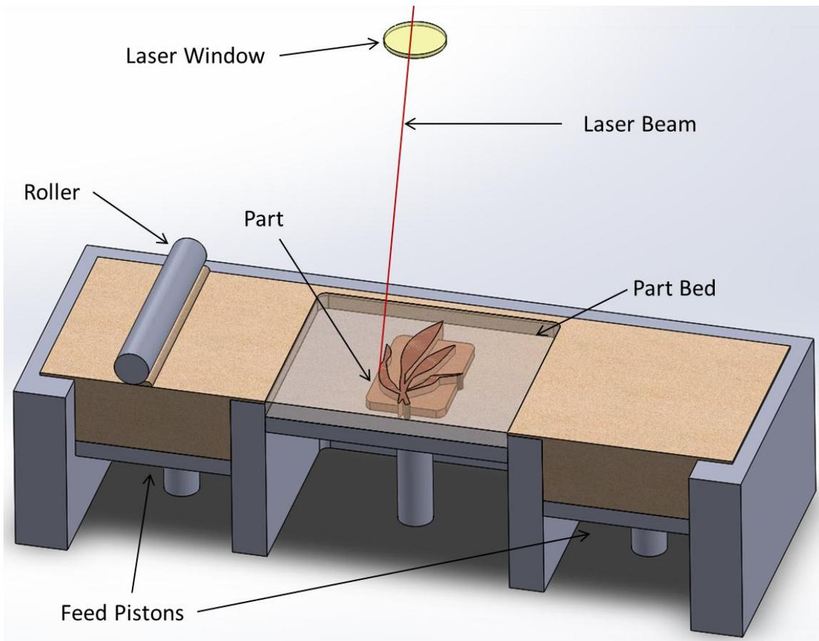
**Figure 1.** *LS machine schematic; laser window and beam*
