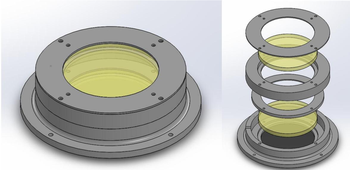
**Figure 6.** *CAD images of modified laser window housing*
