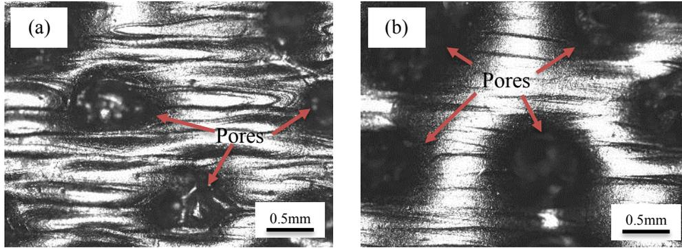
Fig. 16 Top Surface of EBM Specimens (a) LO=0.26mm and (b) FO=20mA
