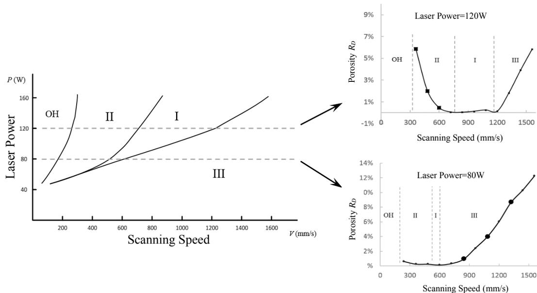
Fig. 1 Process Window of SLM and Porosity Distribution at 120W and 80W
