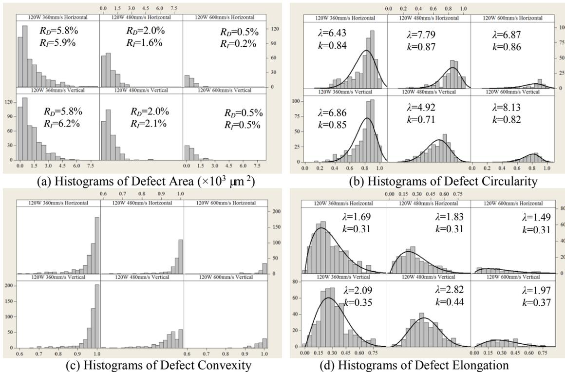
Fig. 6 Distribution of Defect Morphology of SLM-produced Zone II Specimen
