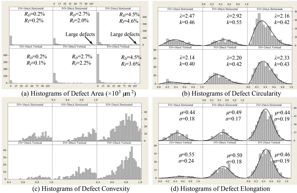
Fig. 15 Distribution of Focus Offset Defect Morphology of EBM-produced Specimens
