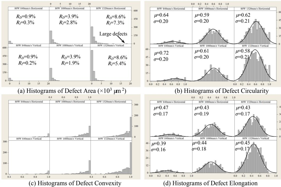
Fig. 8 Distribution of Defect Morphology of SLM-produced Zone III Specimen
