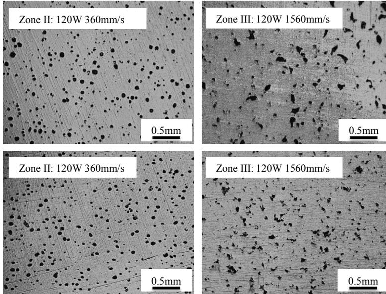
Fig. 9 Cross Section of SLM-produced Specimen (120W 360mm/s vs. 120W 1560mm/s)
