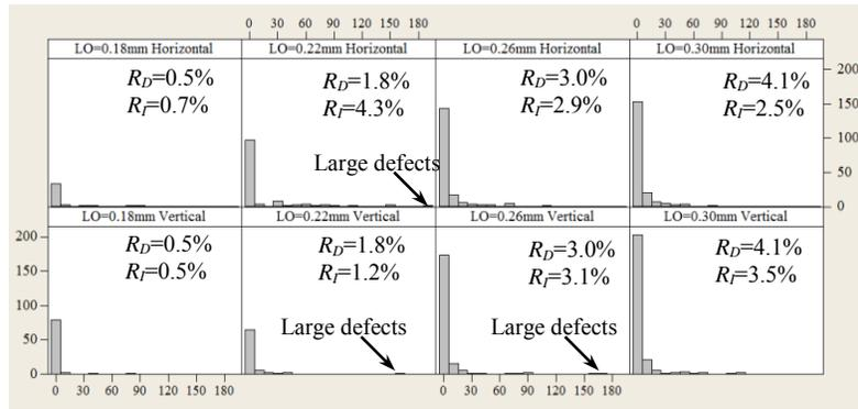
(a) Histograms of Defect Area ( $\times 10^3 \mu\text{m}^2$ )
