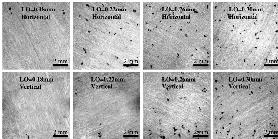
Fig. 12 Cross Sections of EBM-produced Specimen at Various Line Offset Values
