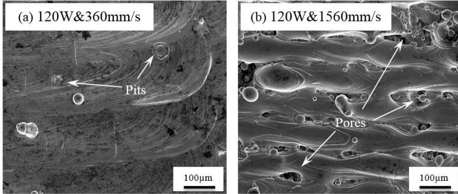
Fig. 11 Top Surfaces of SLM Specimens by Marginal Parameters (a) Zone II and (b) Zone III
