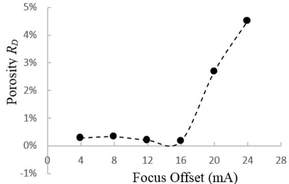
Fig.3 EBM Porosity versus Focus Offset
