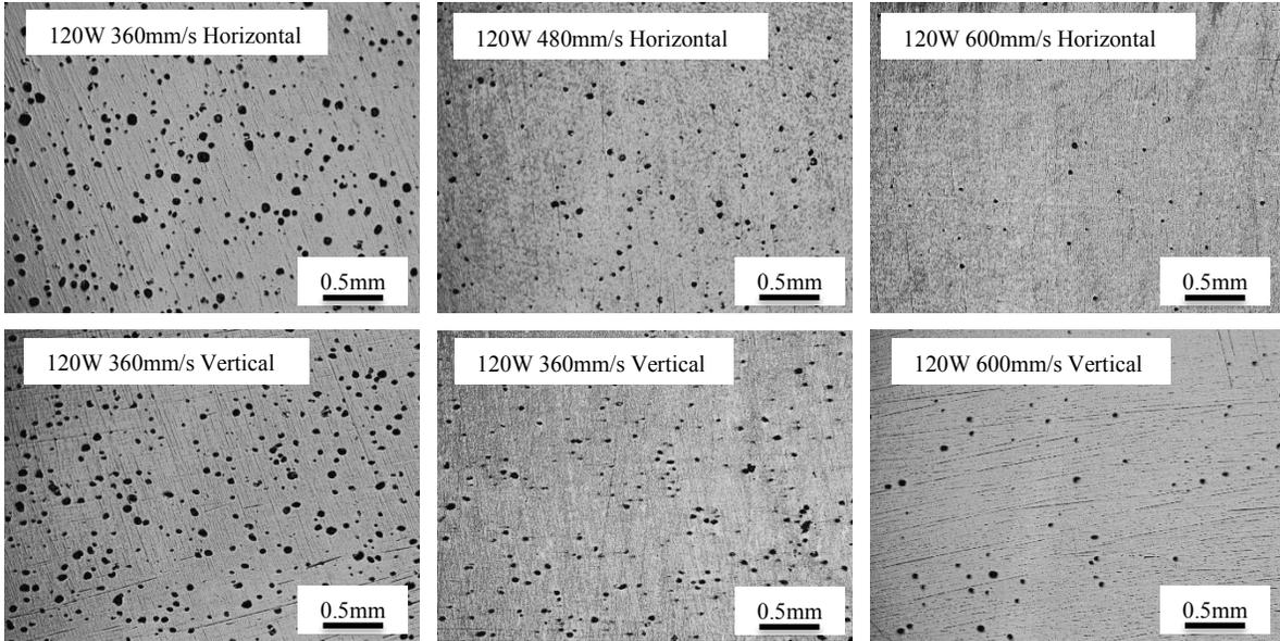
Fig. 5 Cross Section of SLM-produced Zone II Specimens
