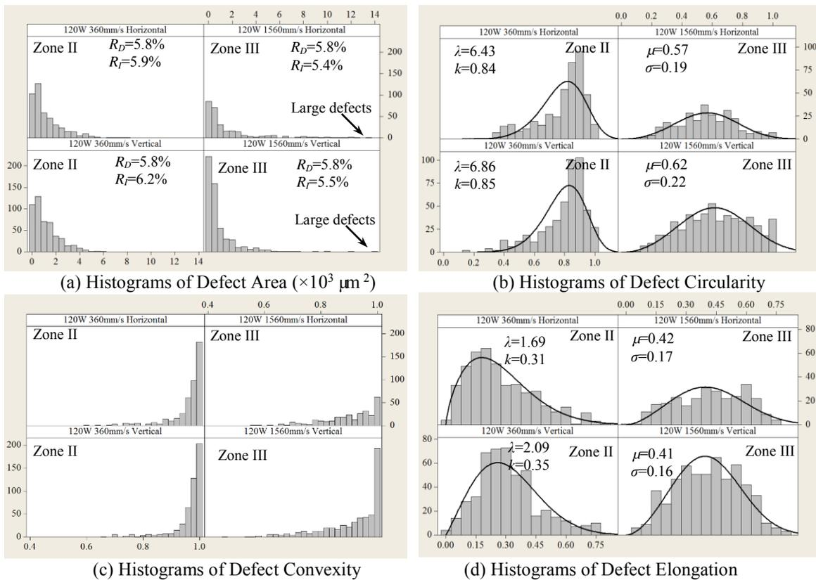
Fig. 10 Distribution of Defect Morphology of SLM-produced Zone II and III (Porosity $\approx$ 5.8%)
