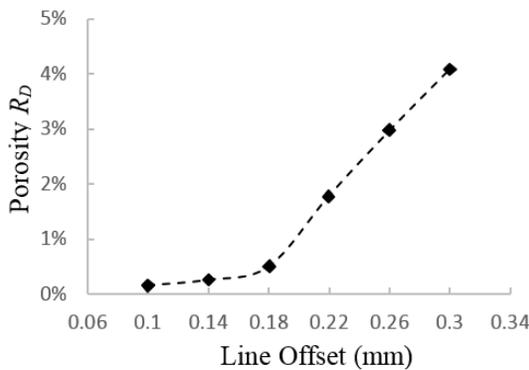
Fig.2 EBM Porosity versus Line Offset
