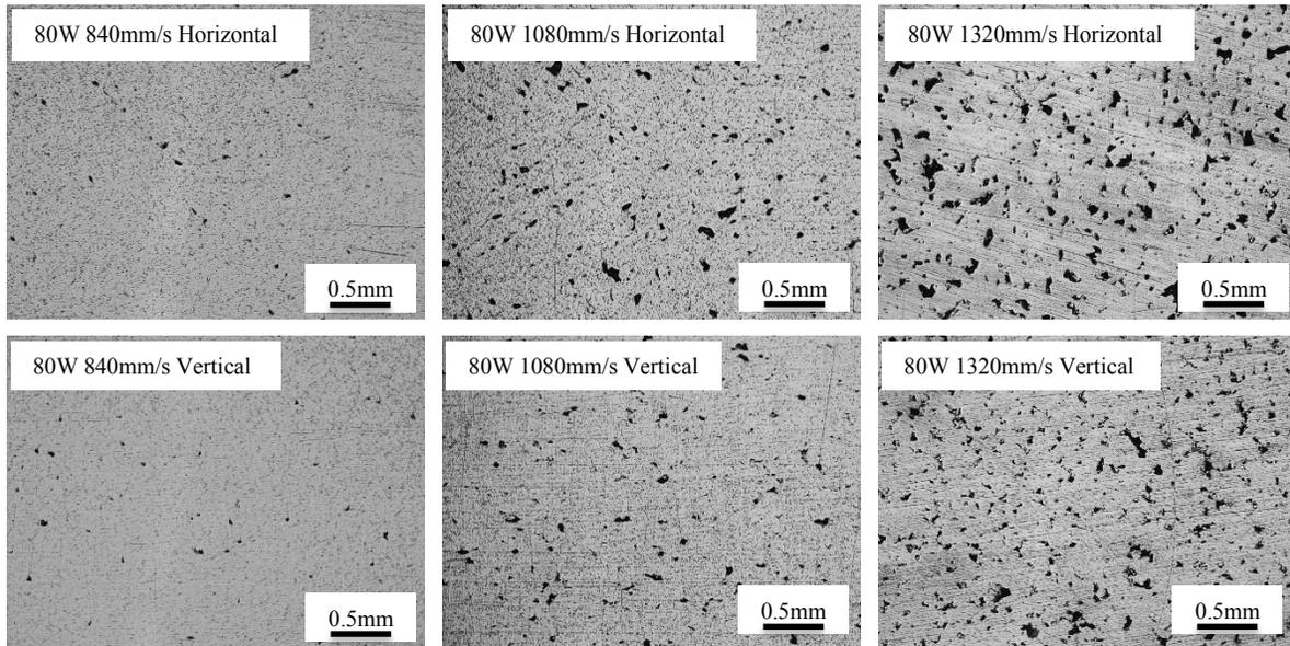
Fig. 7 Cross Section of SLM-produced Zone III Specimens
