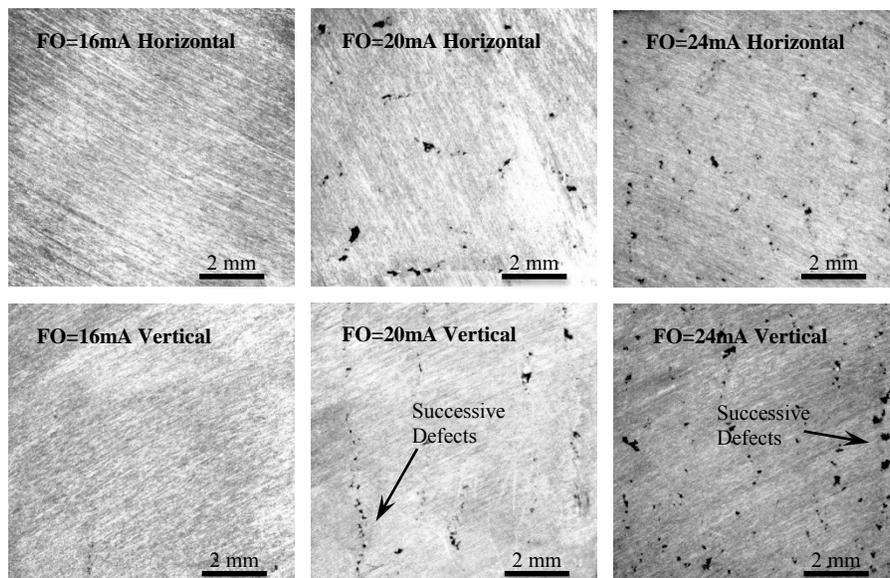
Fig. 14 Cross Sections of EBM-produced Specimen at Various Focus Offset Values
