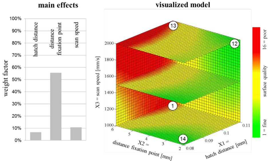
Figure 7: Main effects on surface quality (left); visualized model (right)
