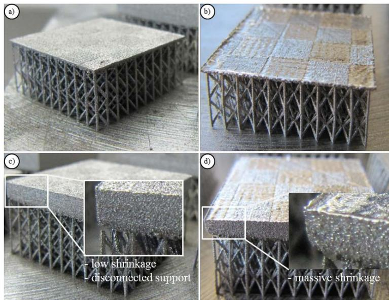
Figure 9: a) 20 connection layers (parameter set 12); b) 20 connection layers (parameter set 14)
