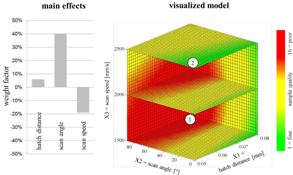
Figure 11: Main effects on surface quality (left); visualized model (right)
