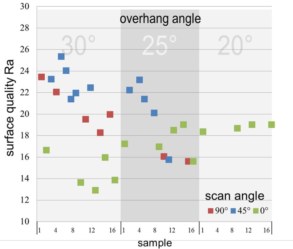
Figure 12: surface qualities (scan angle; overhang angle)
