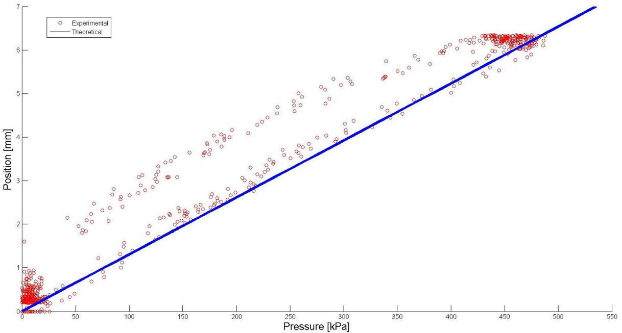
**Figure 8: Toroidal FFA position as a function of internal pressure.**
