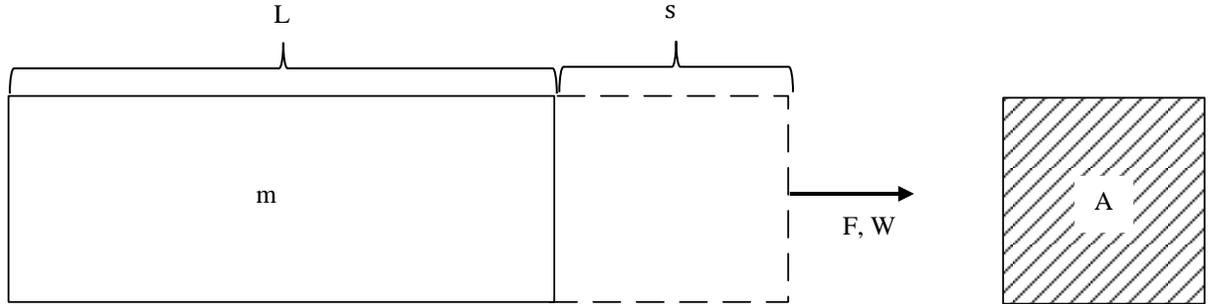
**Figure 5: Free body diagram of a general actuating element.**
