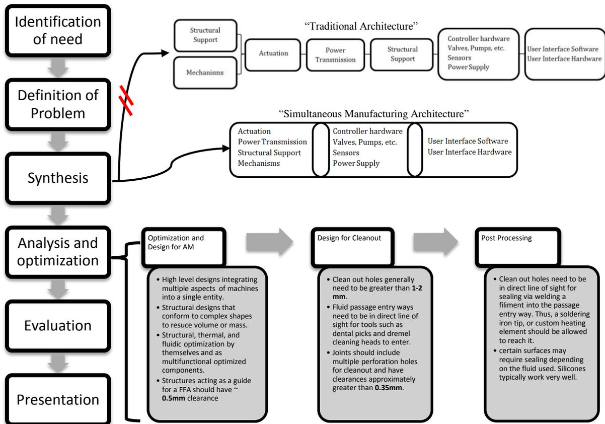
**Figure 3: Simultaneous manufacturing architecture and design outlines [21].**
