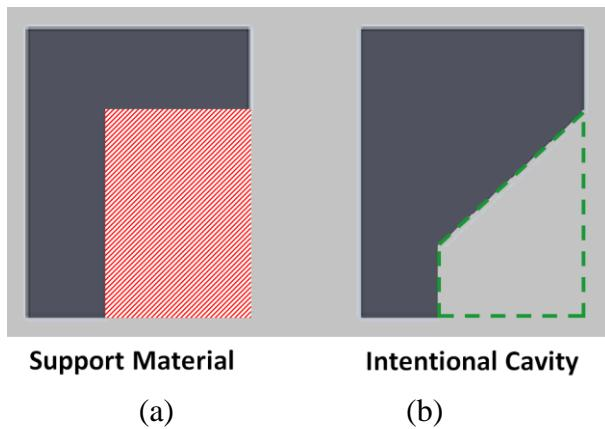
*Figure 1 – Design comparison (a) support needed (b) no*
