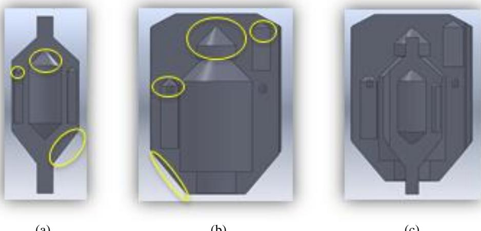
*Figure 3 –CAD file (a) rotor (b) stator (c) full drawing, showing cavities with "roofs", highlighted in yellow are 45 degree features eliminating the use of sacrificial material*
