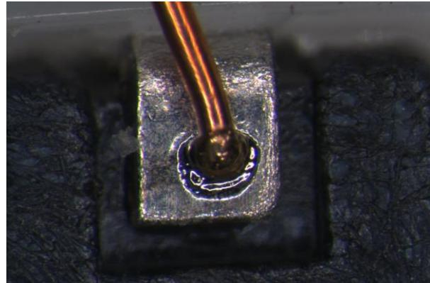
Figure 6 – Micro-Welding with YAG laser
