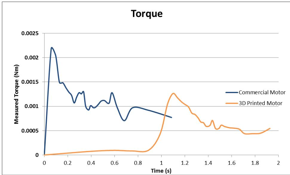
*Figure 9 – Torque comparison*
