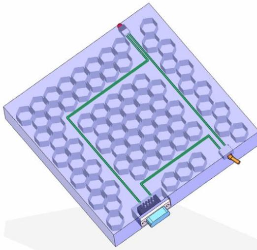
**Figure 1 – Cross sectional view of embedded circuit in honeycomb structure fabricated with the hybridization of UC and DW [5]**
