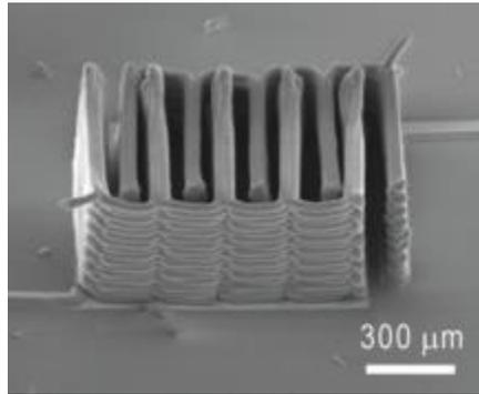
**Figure 3 – SEM images of additively manufactured battery electrode [11]**
