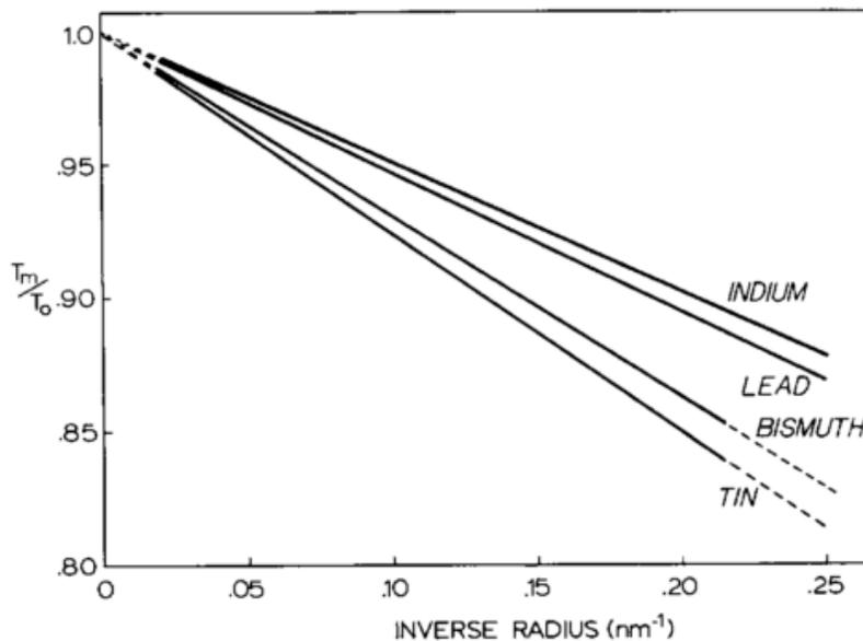
**Figure 8 – Melting temperatures as a function of particle radius demonstrating lowered melting temperatures as size decreases [26]**
