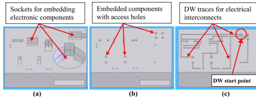
**Figure 13 – Build stages for DW and SLA incorporating vertical interconnects. (a) sockets for embedded components; (b) vias to access embedded components (c) planar interconnects [15]**
