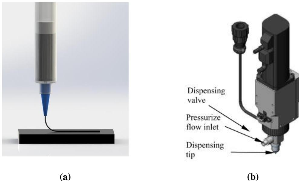
**Figure 5 – (a) schematic of basic syringe system (b) micro-dispensing pump [16]**
