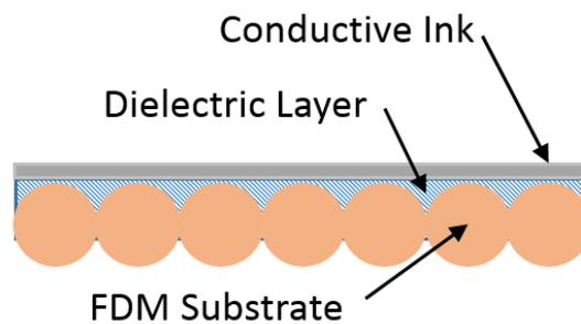
**Figure 12 – Conductive ink deposited on FFF substrate using dielectric intermediate bonding layer**
