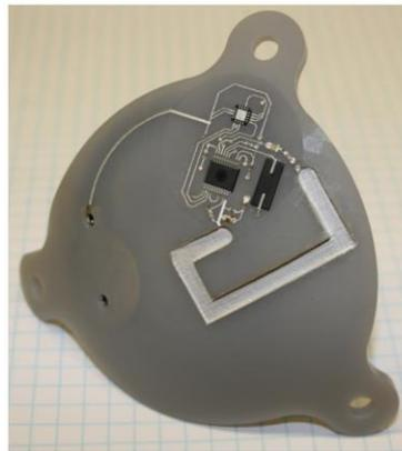
**Figure 2 – Helmet insert for detecting traumatic head injury [8]**
