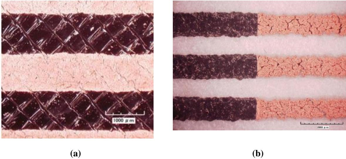
**Figure 10 – Photonic curing of copper on (a) FFF and (b) SLS substrates. (b) Also shows an intentionally uncured region in black [31]**
