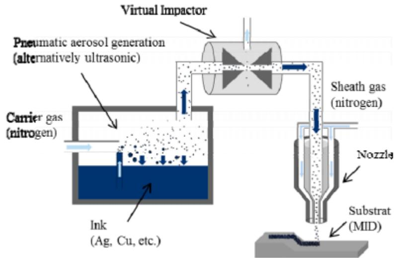
**Figure 7 – Optomec Aerosol Jet process [25]**
