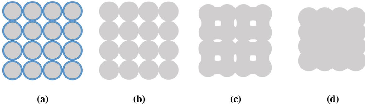
**Figure 9 – Different stages of post-processing to improve conductivity of particle-based metal inks**
