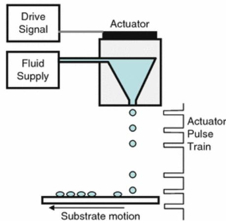
**Figure 6 – Schematic of ink jet deposition [13], [20]**
