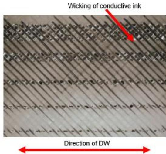
**Figure 11 – Close up image of silver inks deposited on FFF ULETM 9085 printed substrate [35]**
