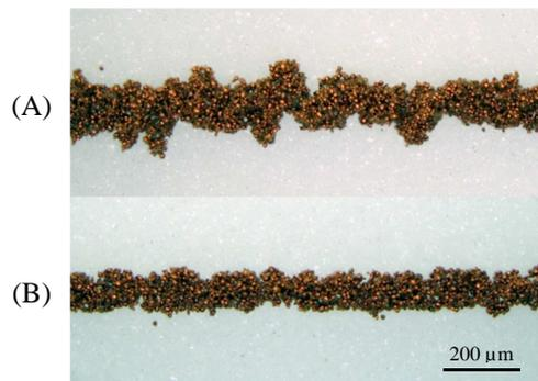
Figure 7 Patterns obtained from two printing conditions with the same nozzle diameter (70  $\mu\text{m}$ ) and the same signal voltage (2 Volts): (A) the standoff distance is 475 $\mu\text{m}$ , and the moving speed is 10 mm/s, (B) the standoff distance is 125  $\mu\text{m}$  and the moving speed is 15 mm/s.
