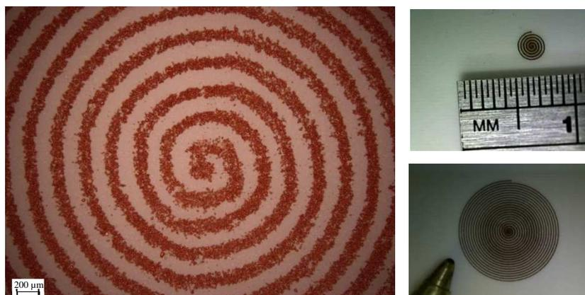
Figure 8 Samples with a track width of less than 100  $\mu\text{m}$ .
