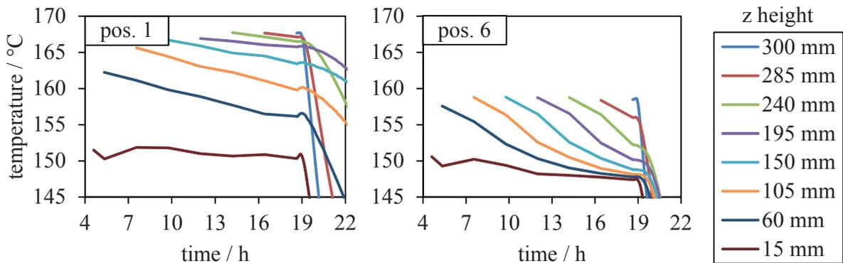
Figure 5: Calculated temperature profile for fixed positions within the part cake during build
