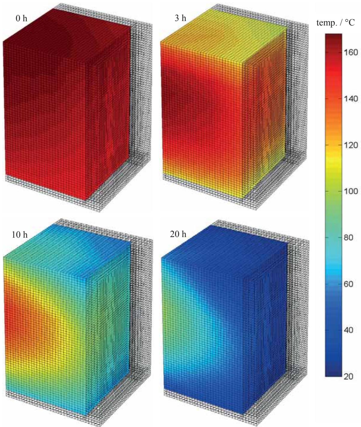
Figure 8: 3D plots of the measured temperature distribution during the cooling process
