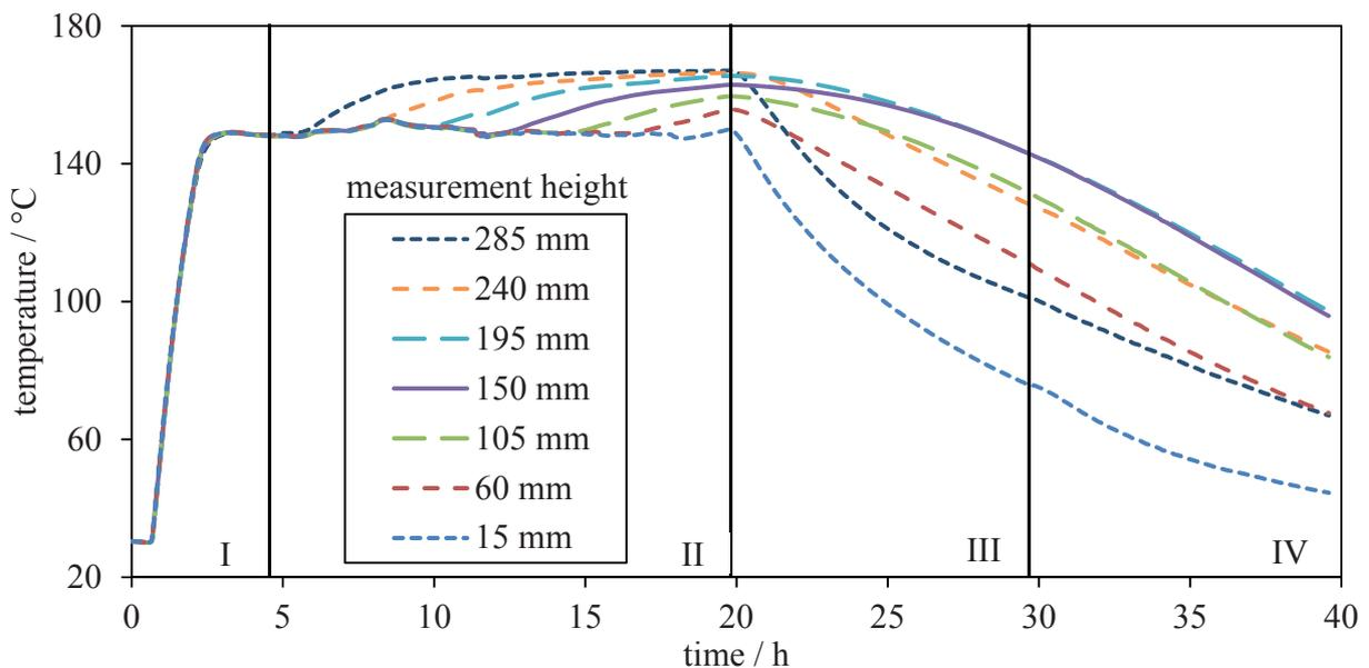
Figure 4: Temperature profile for the (center) sensor bar 1 at different z heights
