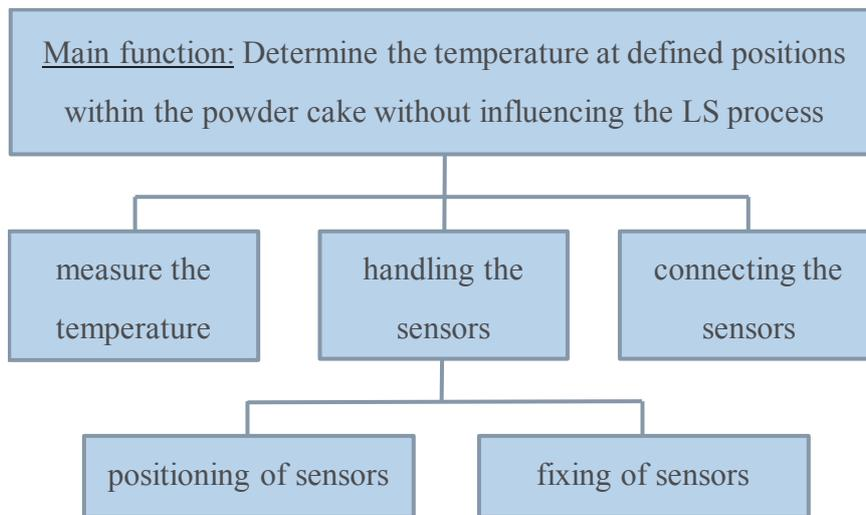
Figure 1: Structured (sub-) functions of the temperature measurement system
