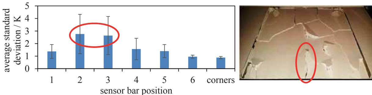
Figure 6: Average standard deviation from test job 1 to 3 during the cooling phase (left) and cracks on the part bed surface (right)
