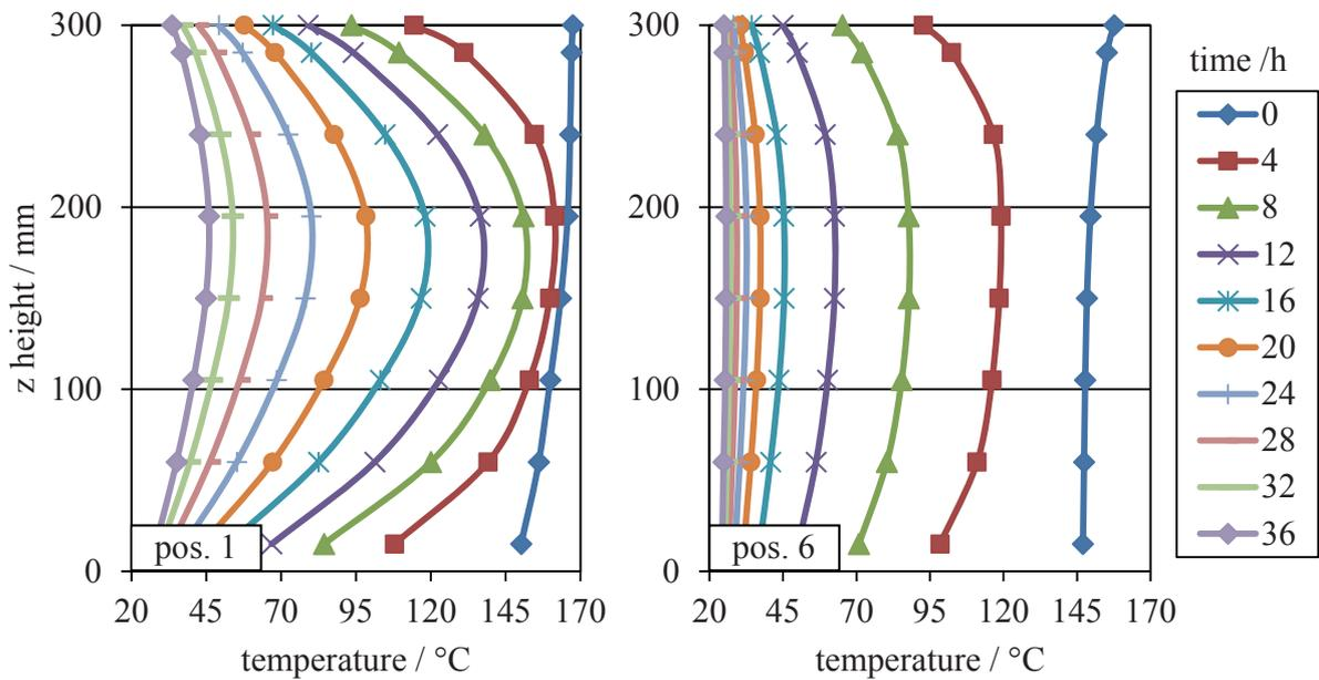
Figure 7: Time dependent temperature profile along the z axis for the sensor bar positions 1 and 6 during the cooling process starting at  $t = 0$  h
