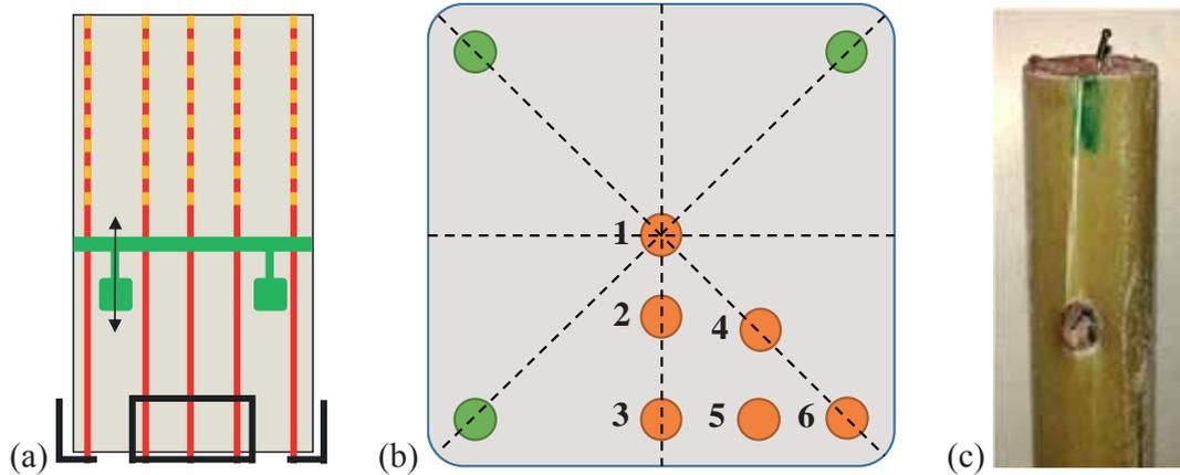
Figure 2: (a) schematic sketch, (b) sensor bar positions, (c) close-up photo of a sensor bar
