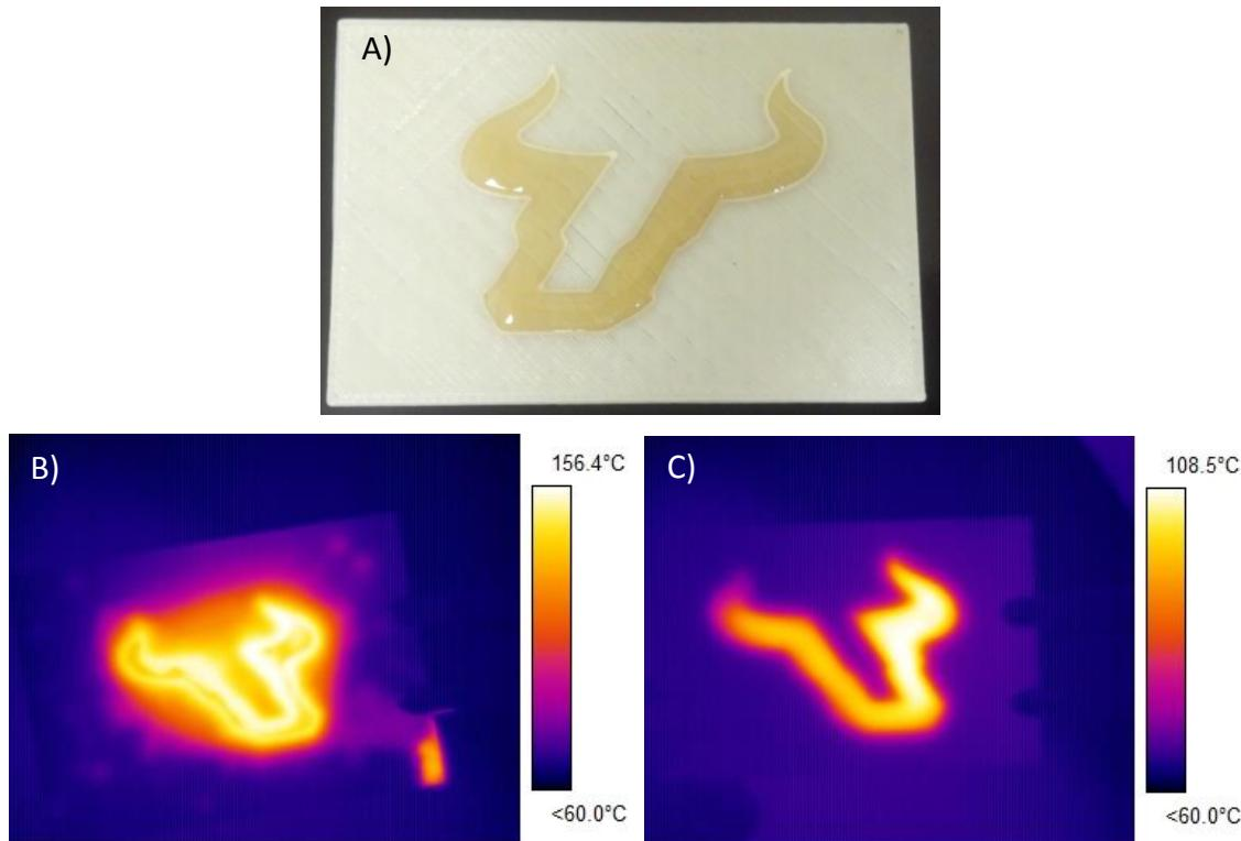
**Figure 6** Microwave heating is used to selectively heat only the desired areas filled with honey. **A)** Part as printed, Thermal image of part from the bottom after microwaving for **B) 45 seconds at 20%** power and **C) 30 seconds at 30%** power in a 900W microwave oven.
