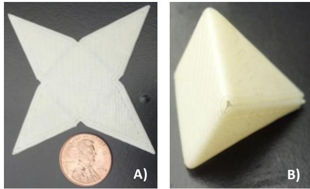
**Figure 2 a)** Part as printed in ABS with parallel horizontal layers **b)** After deformation performed with a pencil torch, layers are aligned into folded directions.
