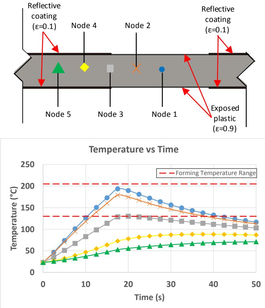
Figure 5 shows the FEA node locations and temperature profile for a joint heated on the top and bottom side by radiation for 17.5 seconds then allowed to cool at room temperature. Only the joints are exposed to the infrared radiation while a copper coating on the structure of the component reflects away unwanted radiation.
