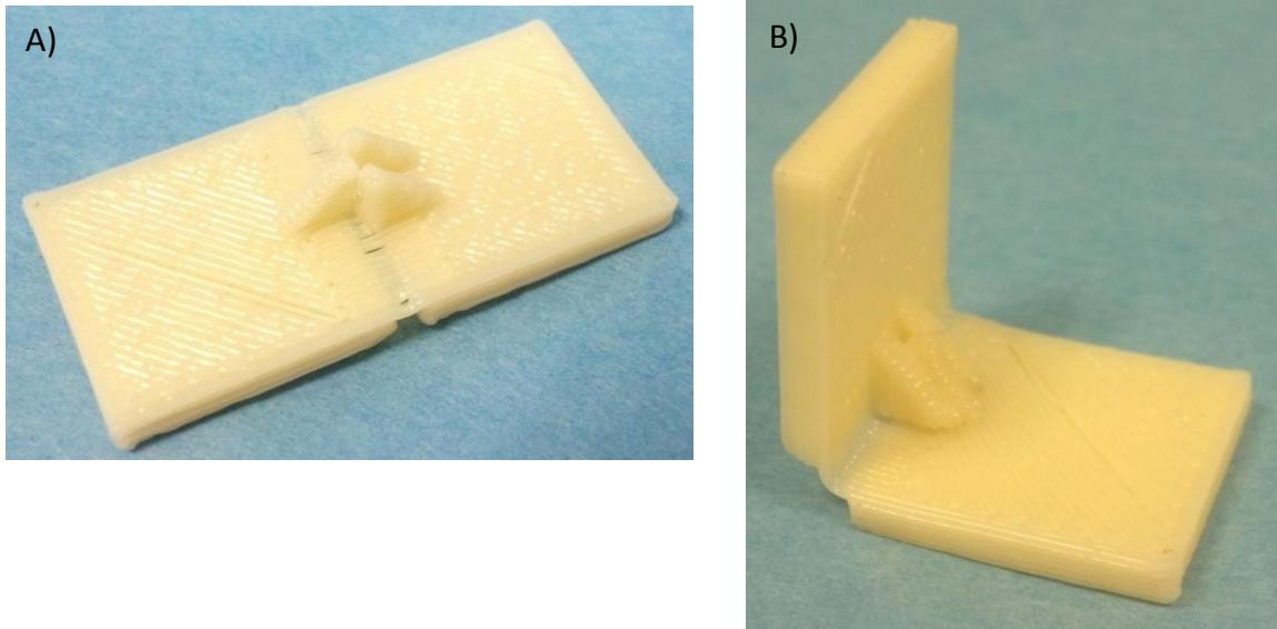
**Figure 7 Surface mounted angle lock. A) Before deformation B) After deformation.**
