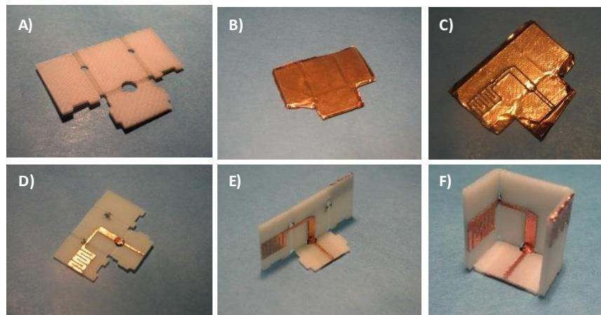
**Figure 1 Formation of 3D printed Antenna. A) Part as printed B) Component coated with copper tape C) Electrical paths cut into copper D) Excess tape removed E) Deformation F) Final Component [2]**
