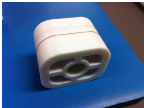
Fig10. wire embedded air flow duct
