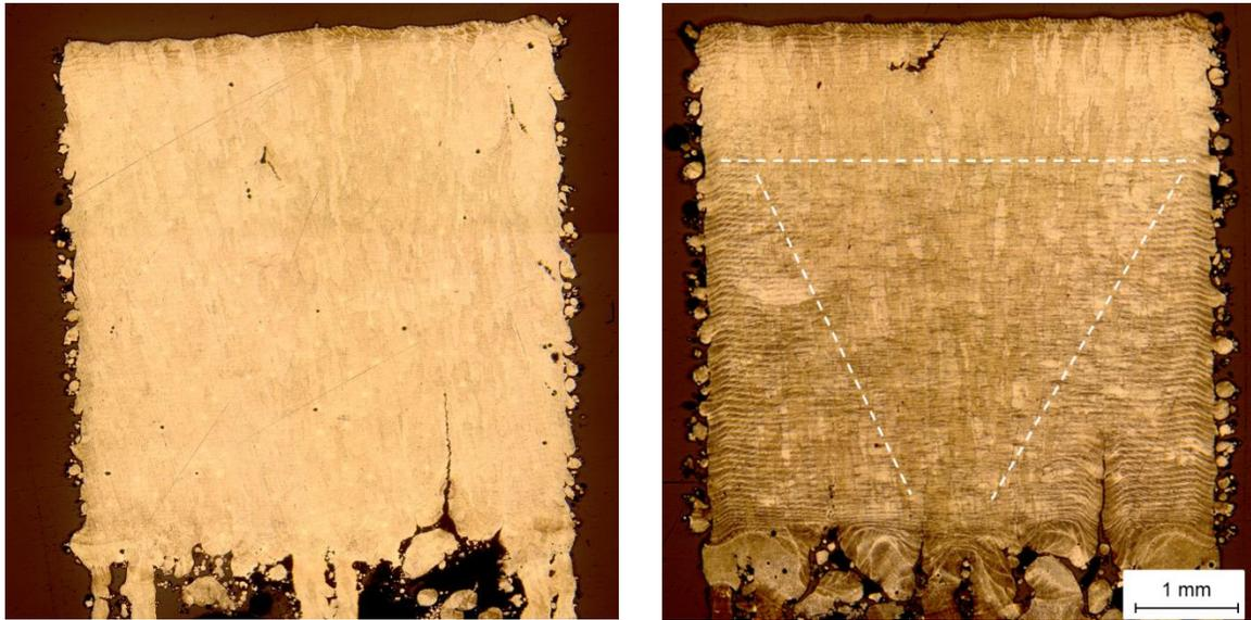
Fig. 10 Etched microsections of cubes on supports, left AW-2022, right AW-2024
