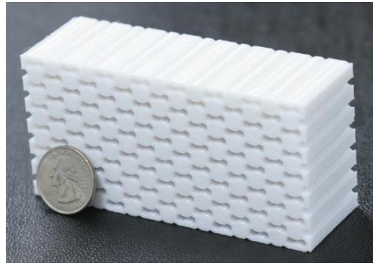
**Figure 1. 3D printed anisotropic metamaterial [28].**
