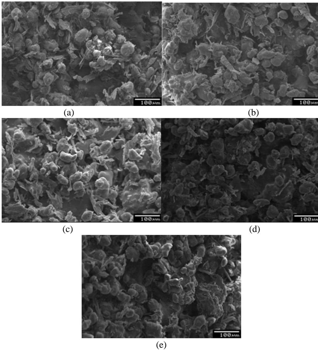
Fig. 8 SEM photos of EPA 12 part surfaces magnified by 200 times (a) built by 10 W of laser power; (b) built by 15 W of laser power; (c) built by 20 W of laser power; (d) built by 25 W of laser power; (e) built by 30 W of laser power
