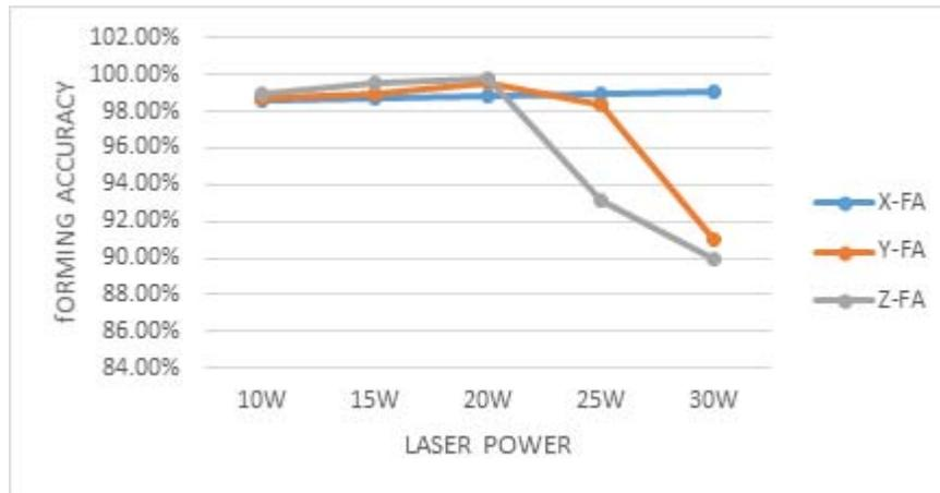
Fig. 6 Forming accuracy of laser sintered EPA12
