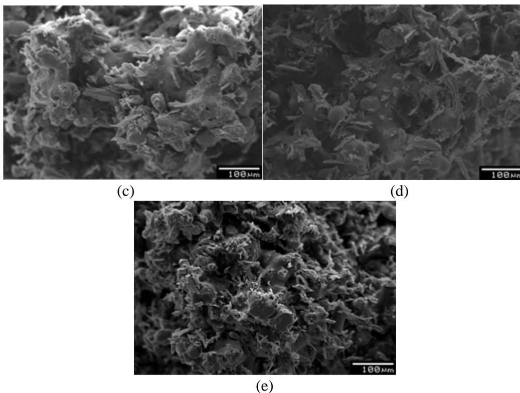
Fig. 8 SEM photos of EPA 12 part cross-sections magnified by 200 times (a) built by 10 W of laser power; (b) built by 15 W of laser power; (c) built by 20 W of laser power; (d) built by 25 W of laser power; (e) built by 30 W of laser power
