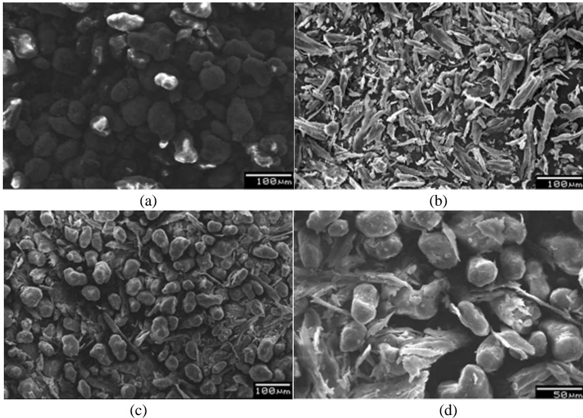
Fig. 3 SEM Micrographs of (a) Neat PA 12 magnified by 200 times (b) Neat eucalyptus powder magnified by 200 times (c) blend magnified by 150 times (d) blend magnified by 400 times
