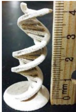
Fig.5 Demonstration part processed using DTM Sinterstation HiQ® (Laser Power: 24 W, Scanning Speed: 2000 mm/s, Scanning Space: 0.15 mm, Layer Thickness: 0.127 mm, Part Bed Temperature: 174 °C) in Ratio of 1:2 eucalyptus/PA12
