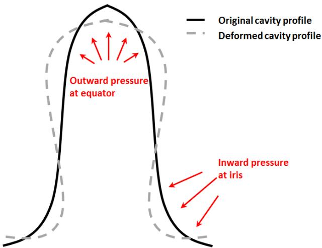
**Figure 3 – Lorentz forces acting in the wall of an SRF cavity causing its deformation.**
