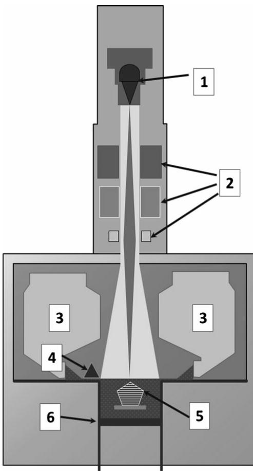
**Figure 1 – Schematic of the Arcam electron beam melting system**
