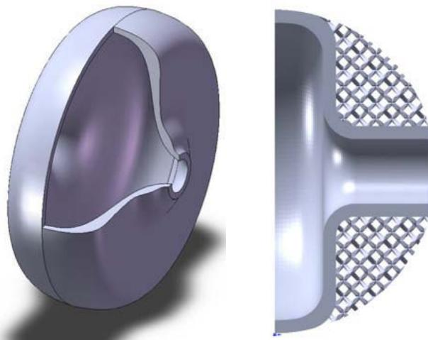
**Figure 4 – CAD rendering of the cavity profile with varying thickness and integrated support structures to the wall of a cavity**
