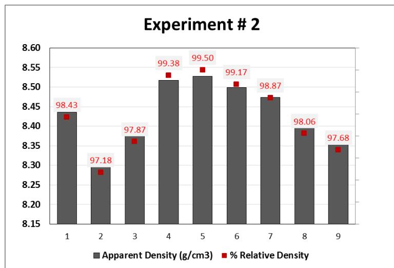
Figure 10 – Results for density measurements in experiment 2.
