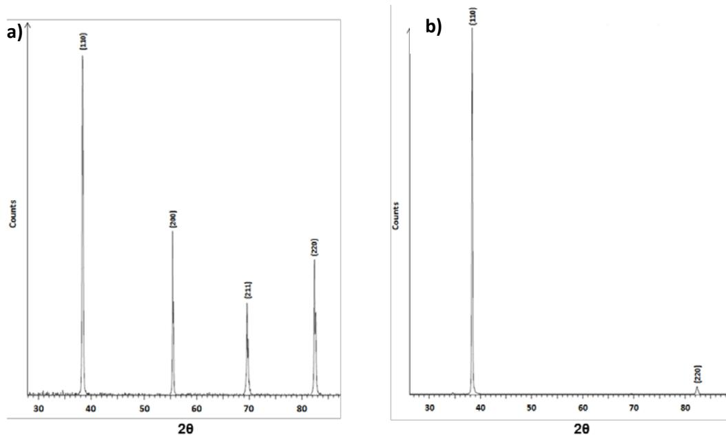
**Figure 15 – XRD spectra for a) powder and b) EBM niobium specimens**
