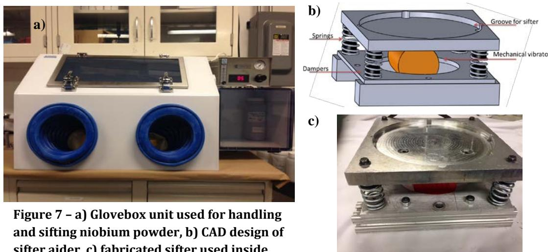
**Figure 7 - a) Glovebox unit used for handling and sifting niobium powder, b) CAD design of sifter aider, c) fabricated sifter used inside glovebox.**
