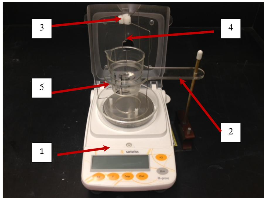
**Figure 6 -Weight balance and density measurement kit used for EBM niobium parts.**
