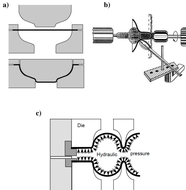
**Figure 2 – Traditional fabrication methods for SRF cavities. a) deep-drawing, b) spinning and c) hydroforming.**
