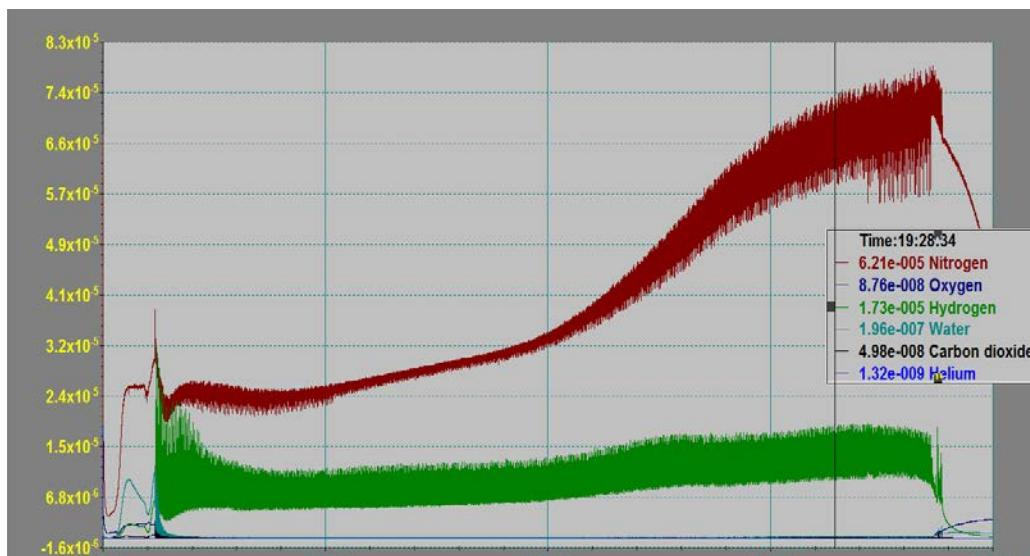
Figure 14 - Typical RGA plot observed during fabrication with niobium.
