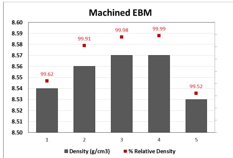
Figure 12 – Measured apparent and percent relative densities for EBM part with machined edges.
