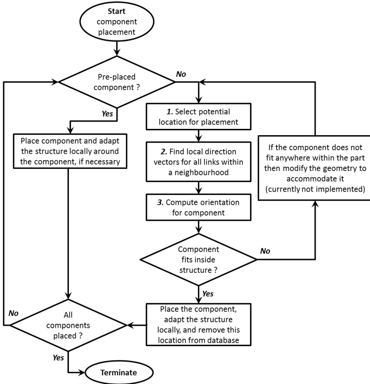
Figure 6: The placement methodology
