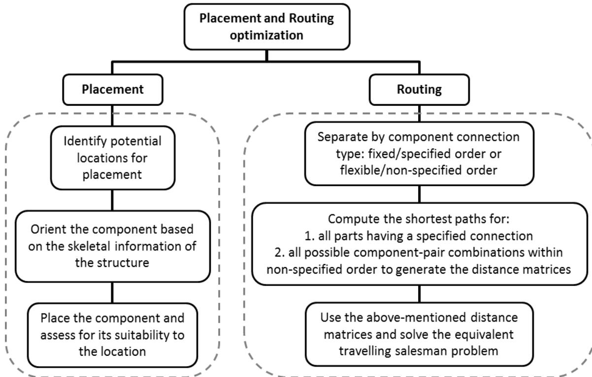
Figure 4: Description of the placement and routing strategy.
