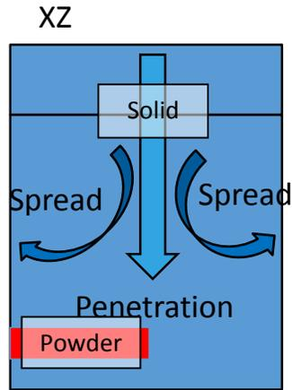
Figure 9: Inhomogeneous case in the -z direction showing a solid part with an internal cavity and entrapped powder
