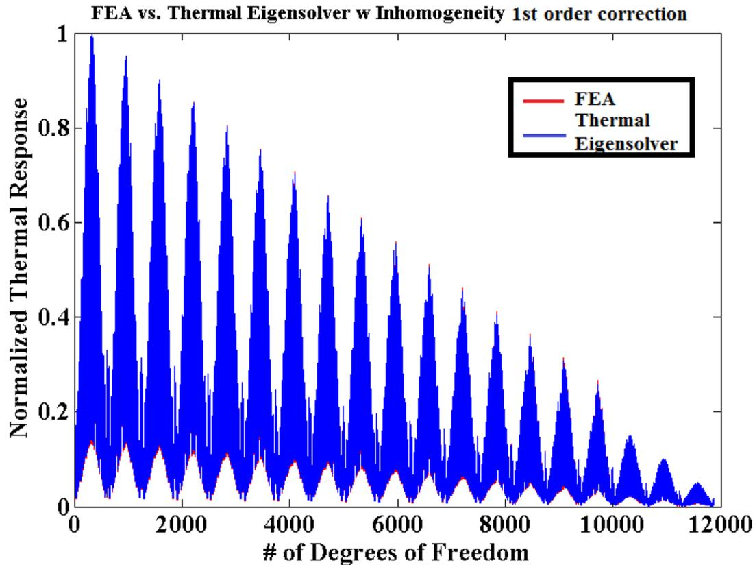
Figure 10: FEA and Thermal eigensolver with 1st order correction one-on-one DOF comparison using homogenous modes for computation.
