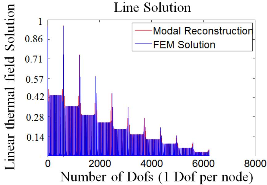
Figure 6: Nodal Point by point comparison of a finite element solution with a Modal reconstructed solution for a constant line energy source. The match is good but not excellent when compared to Figure 5.
