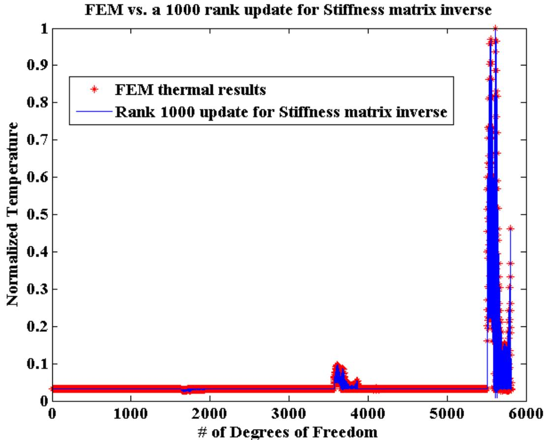
Figure 12: Thermal distributions computed by performing the LU/Cholesky Decomposition of the full thermal stiffness matrix against a much lower rank update of the inverse.
