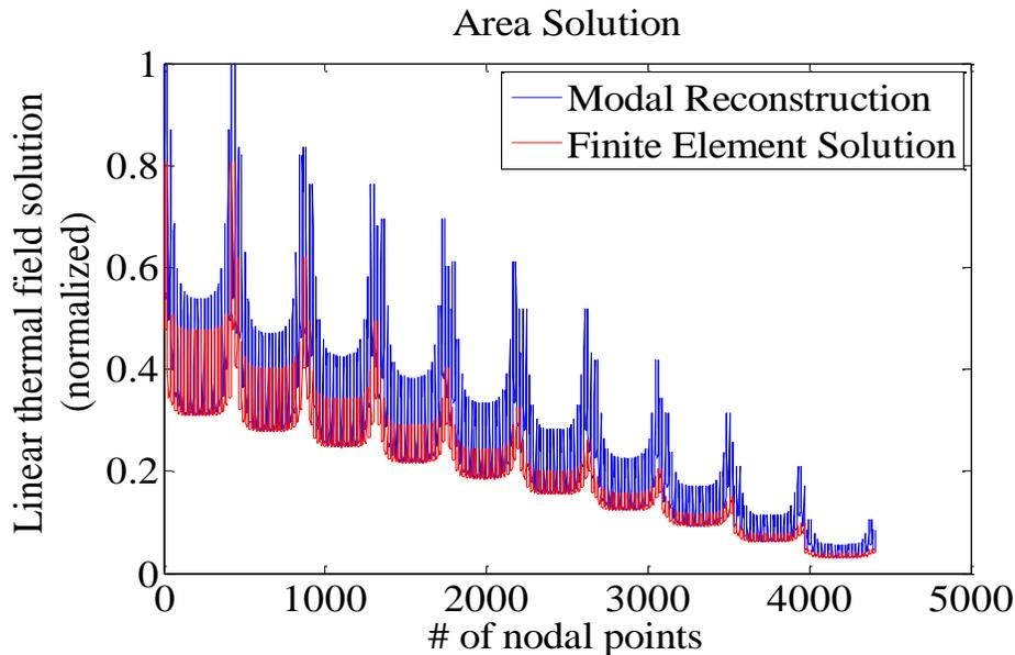
Figure 7: Nodal Point by point comparison of a finite element solution with a Modal reconstructed solution for an area energy source. The modally reconstructed solution matches the trend but not the magnitude of the solution due to unrefined orthogonal modes. This result is irrelevant for moving point energy problems associated with SLM or EBM, but should be taken into account when seeking the correct solution for area energy sources.
