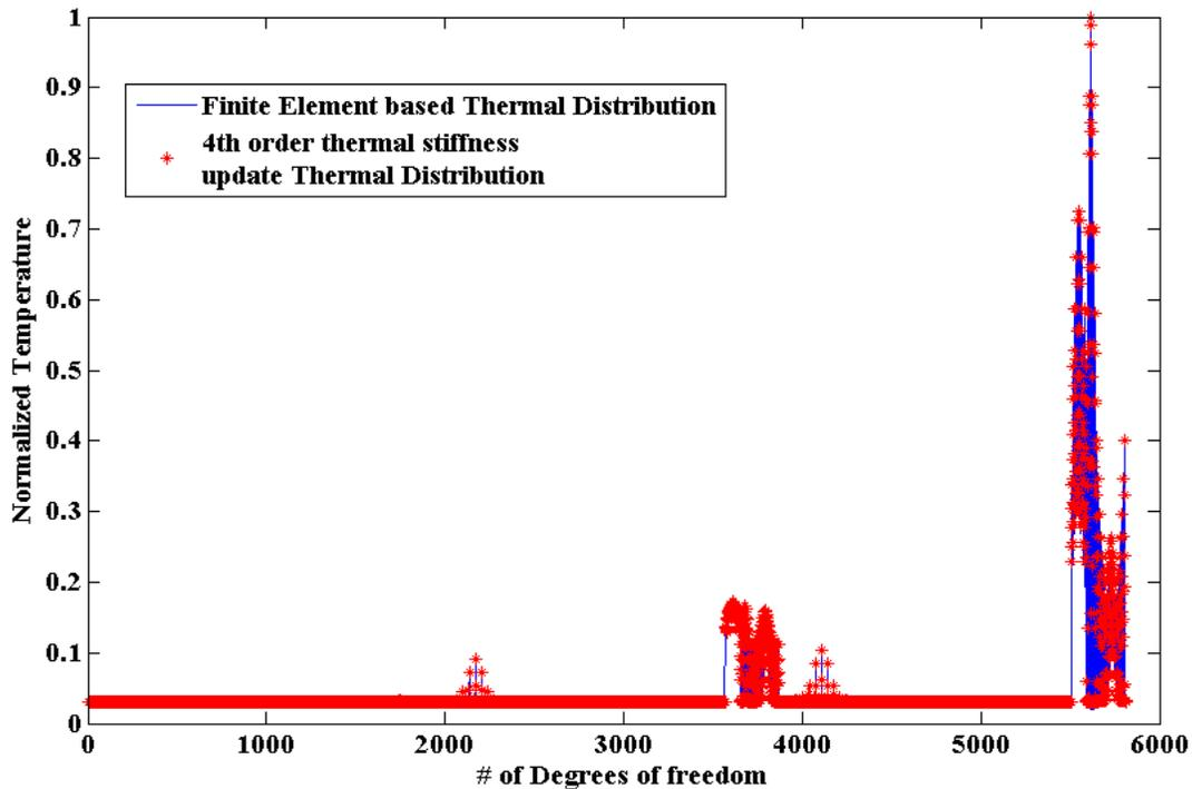
Figure 13: Thermal distributions computed by performing the LU/Cholesky Decomposition of the full thermal stiffness matrix against a much lower order update of the inverse.
