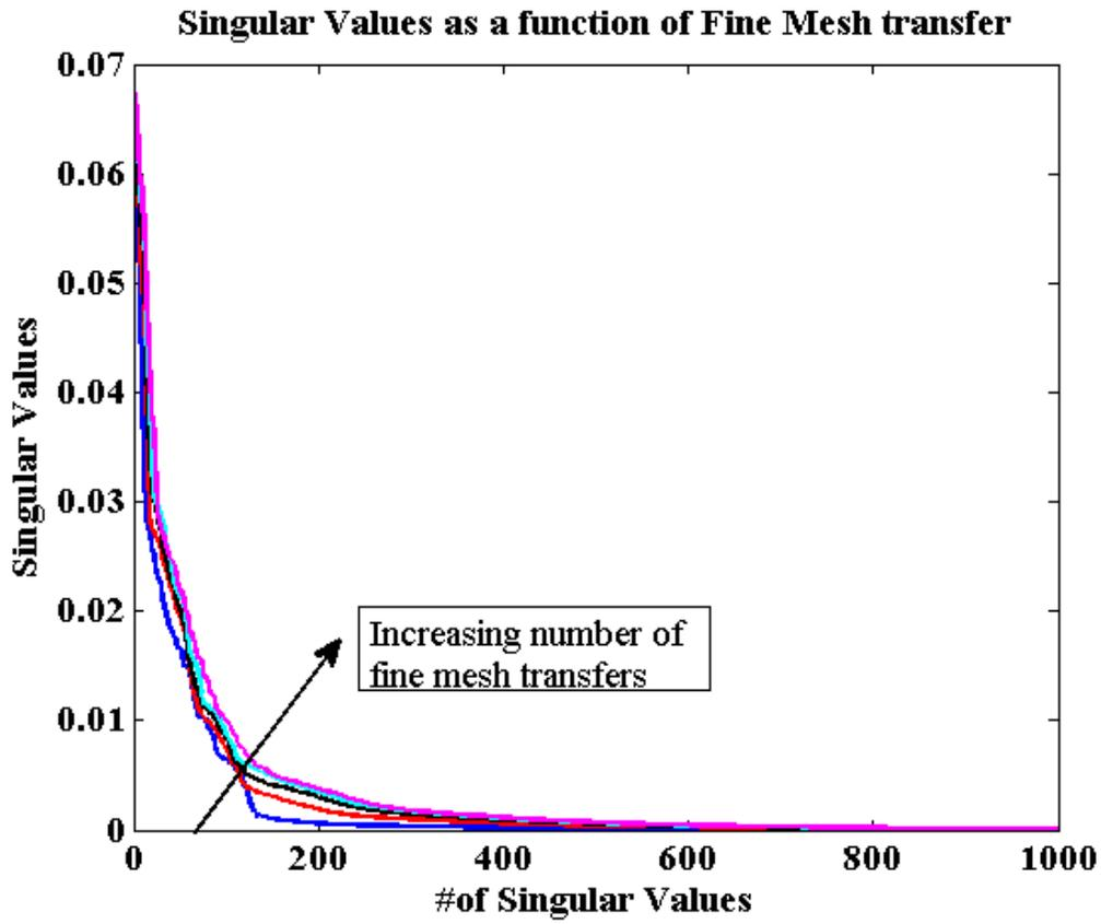
Figure 11: Singular values as a function of fine mesh transfer offsets
