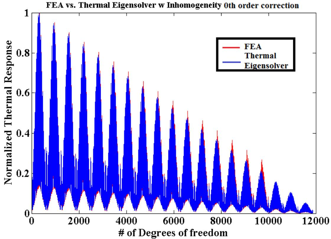
Figure 8: FEA and Thermal eigensolver with 0<sup>th</sup> order correction for node-by-node comparison using homogenous modes for computation
