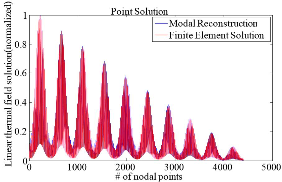
Figure 5: Nodal point by point match of a finite element solution for a thermal field with a Modal reconstructed (eigensolver) solution for a Gaussian point energy source. The error is negligibly small ( $<0.1\%$ ) and the results lie right on top of each other.
