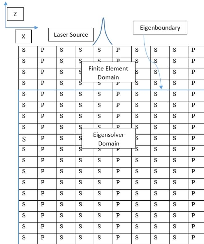
Figure 2: XZ plane cross-section elements viewed from the -Y direction. The Solid-Powder pattern in the +X direction is repeated and extruded in the -Z direction, illustrating a part with the same cross-sectional geometry between layers. S denotes the portion of the powder bed which has converted from powder to solid following laser exposure and P denotes the portion of the powder bed which didn't change its state and remained as powder.
