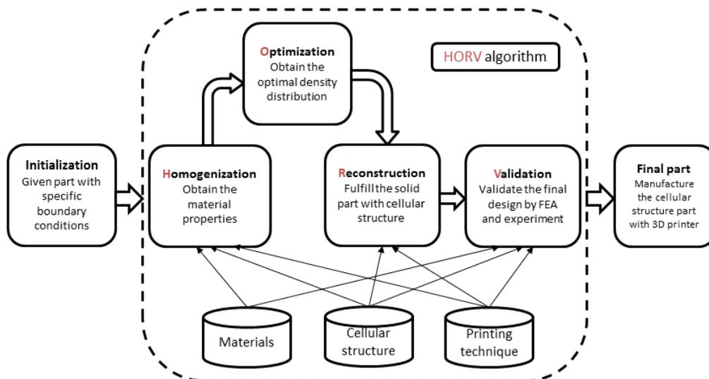
Fig. 1 The flow chart of the HORV algorithm
