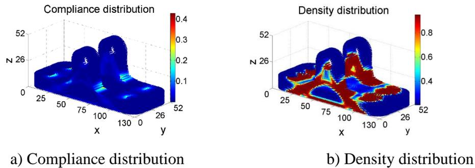
Fig. 5 Topology optimization results of a pillow bracket part with volume fraction as 0.5
