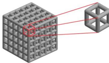
Fig. 2 Assembly of cubic structure and its unit cubic cell
