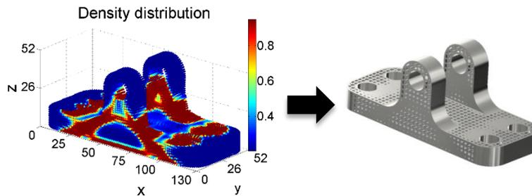
Fig. 6 The reconstruction process for pillow bracket with cubic cellular structure
