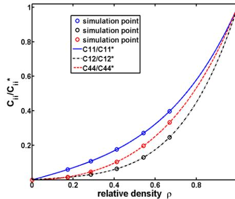
Fig. 3 Elastic scaling laws of cubic cellular structure
