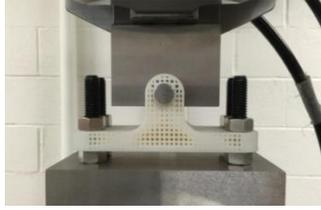
Fig. 7 Experimental setup of the 3-point bending test
