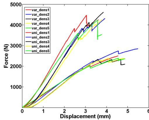
Fig. 8 Testing curves of cubic cellular structure pillow brackets
