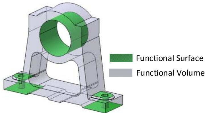
**Figure 2 An example of functional surfaces and a functional volume**
