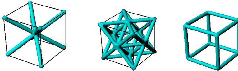
(a) “X” shape lattice      (b) Octet lattice      (c) Square lattice
