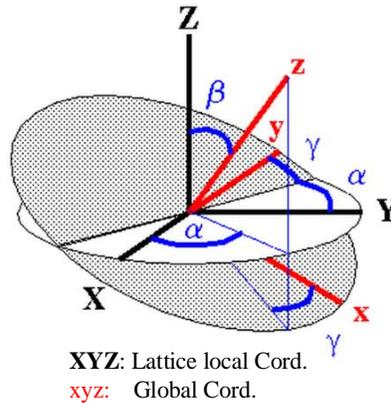
**Figure 5 Relationship between lattice local coordinate and global coordinate**
