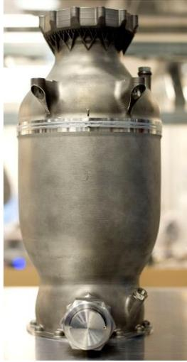
(b) SpaceX combustion chamber [2]
