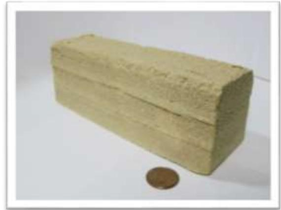
Figure 8: Three layers extrusion sample
