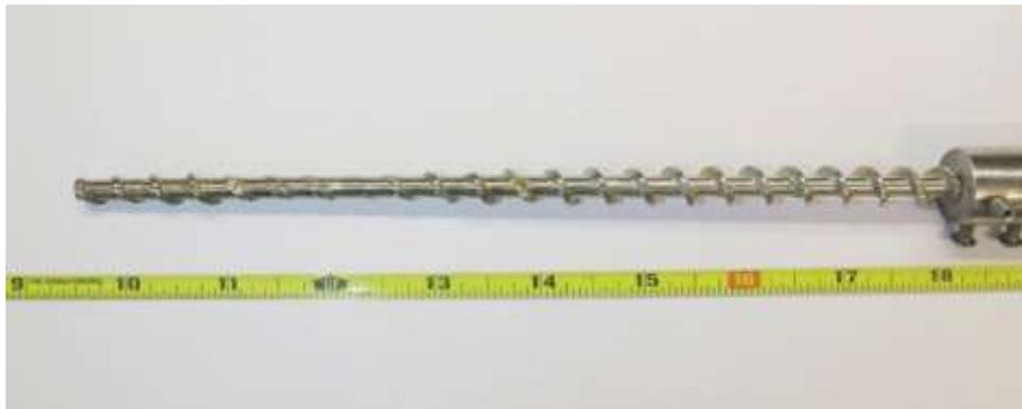
Figure 4: Auger worn-out during experiment
