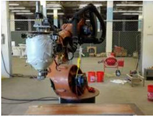
Figure 7: Sulfur concrete contour crafting robot
