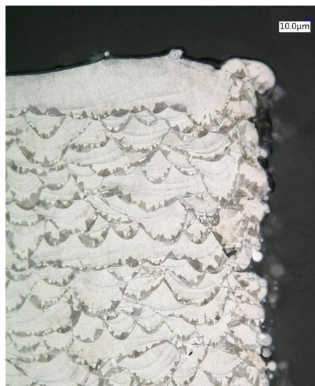
Figure 6: 304L Bulk Sample Imaged at x300
