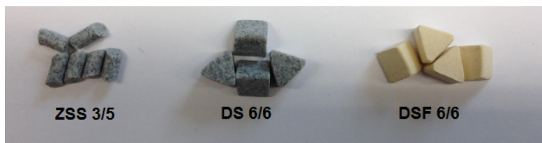
Figure 3: Used grinding media: coarse finish media with cylindric diagonal cut shape and 3 mm and 5 mm edge length (left); coarse finish media with triangle shape and 6 mm edge length (middle); fine finish media with triangle shape and 6 mm edge length (right).
