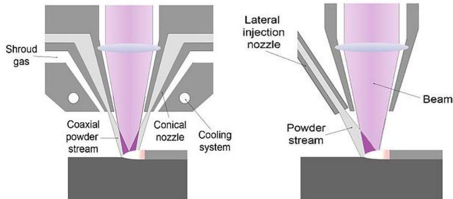
Figure 2 Left is a cross-section sketch of a coaxial blown powder processing head. Right is a cross-section sketch of an off-axis blown powder processing head [5]
