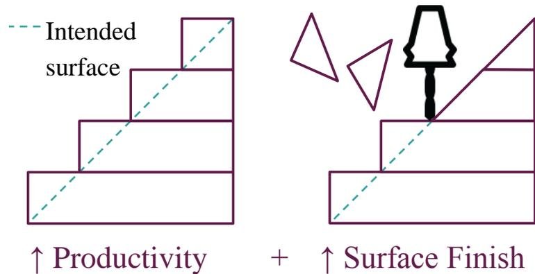
Figure 5 Cross-sectional view showing how an overbuilt part can be machined using the combination of AM and CNC machining [21].
