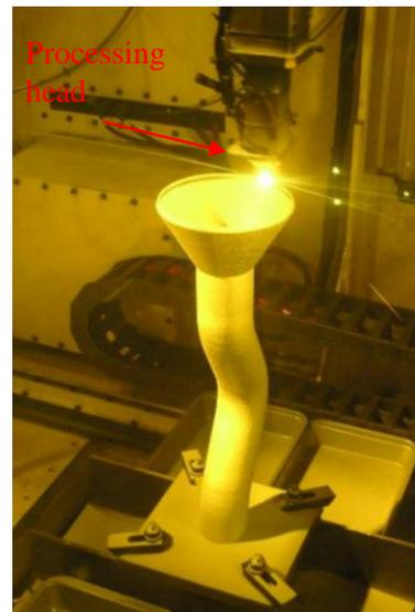
*Figure 4 Left a picture of a fuel cell being built on the Sciaky EBAM machine. Right a picture of a complex automotive component being manufactured on the RPM Solutions machine [18, 19].*
