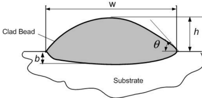
Figure 3 A sketch of a cross section of a typical deposition [10]
