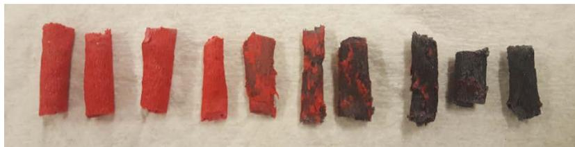
**Figure 5.** Extruded samples transitioning from glass fiber filled ABS (right) to carbon fiber filled ABS (left).
