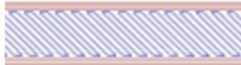
Figure 12: Illustration of gage region toolpaths. Perimeter roads are shown in red; infill roads are shown in blue.
