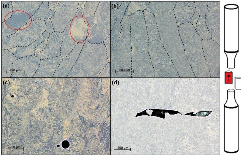
Figure 3. Cross-sectional microstructure of LENS Ti-6Al-4V: (a) single built specimens, (b) double built specimens, and examples of defects found on (c) single built specimens, and (d) double built specimens.
