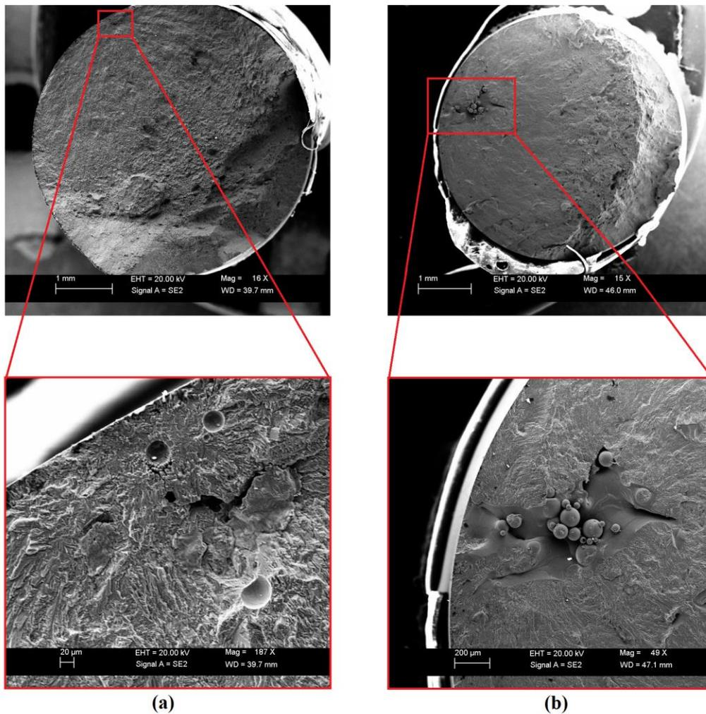
Figure 7. Representative fatigue fracture surfaces for (a) single built and (b) double built LENS Ti-6Al-4V specimens.
