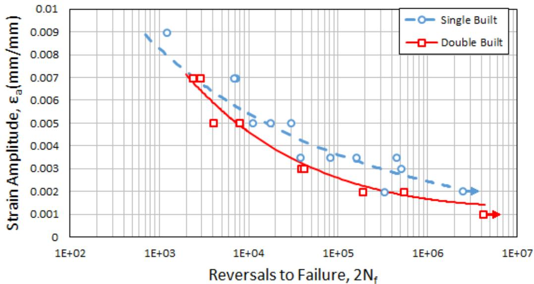
Figure 6. Comparison strain-life fatigue behavior for single and double built LENS Ti-6Al-4V.
