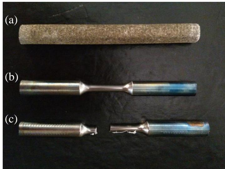
Figure 2. Examples of specimens in the (a) as-built, (b) post-machining, and (c) post-testing state.
