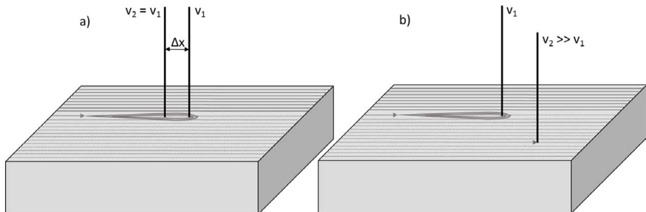
Figure 2: a) Offset strategy: Using two beams in a defined offset at the same speed. b) Heating strategy: Using a melting beam of scan speed  $v_1$  and a heating beam of  $v_2$  which is much faster and irradiates the layer multiple times while beam 1 melts the tracks
