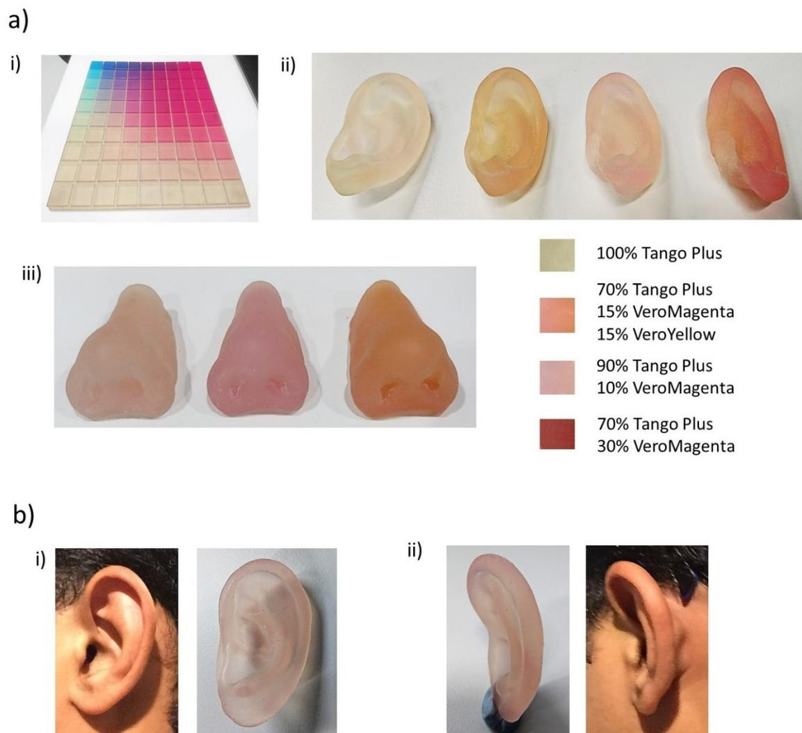
*Figure 5: a) i) An image of the material map which show the various colour combinations possible with the 3D printer using two Vero colours and the flexible Tango plus material, and images of various printed prosthesis of ii) an ear and iii) a nose model. Material combinations are also highlighted in the legend. b) Comparative images of the subject's ear and the 3D printed model from i) side and ii) reverse profiles.*
