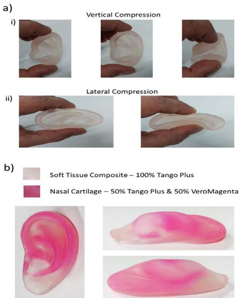
Figure 6: a) Qualitative compression of the model to demonstrate the realism in the tactile feel for both i) vertical and ii) lateral compression. b) Multi-model printing of the ear, with independent material combinations for the cartilage and residual soft tissue composite.
