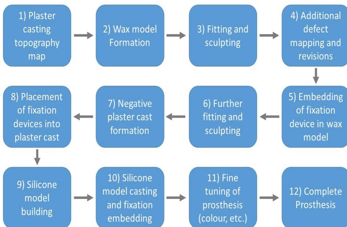
Figure 1: Traditional process chain for prosthesis fabrication
