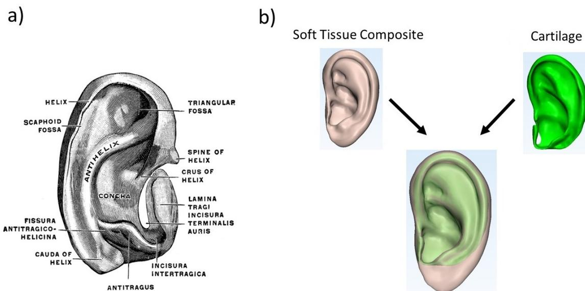
Figure 4: a) A classical medical diagram of the cartilage within the ear [17], adapted from [https://lookfordiagnosis.com/mesh\\_info.php?term=ear+cartilage&lang=1](https://lookfordiagnosis.com/mesh_info.php?term=ear+cartilage&lang=1). b) The multi-model design of the ear prosthesis comprising the soft tissue composite and the cartilage. For visualisation purposes both segments are also represented individually.
