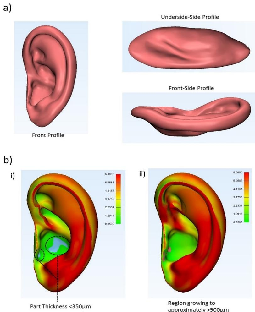
Figure 3: a) Various orientations of the ear prosthesis model. b) Colour map thickness analysis of the ear model for i) the raw data model input from the 3D scanner software, ii) post processed model to grow the thickness of the inner ear section to approximately  $\geq 1\text{mm}$ .
