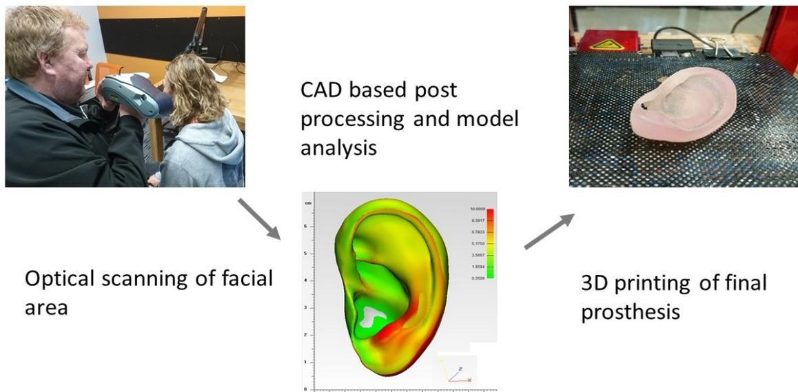
Figure 2: Diagram illustrating the proposed process chain for prosthesis production
