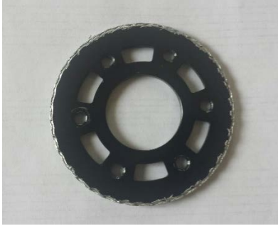
Figure 11: Metal sprocket post fatigue test.
