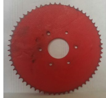
Figure 12: 3D printed sprocket post fatigue test.
