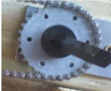
Figure 3: 3D printed sprocket attached to test apparatus.
