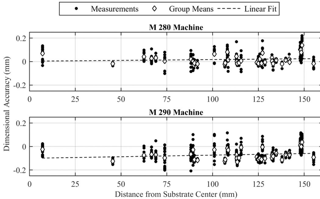
Figure 8: Dimensional accuracy plotted as a function of distance from substrate center to part measurement location.
