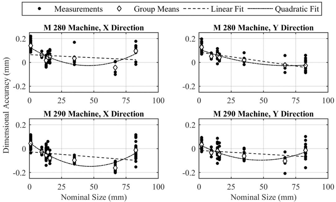
Figure 11: Dimensional accuracy plotted as a function of nominal part size with linear and quadratic regression models fitted to the data. [7]
