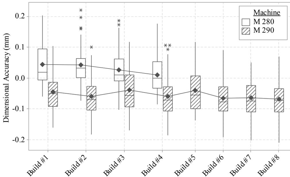
Figure 3: Box and whisker plot comparing dimensional accuracy across multiple AM builds and two AM machines.
