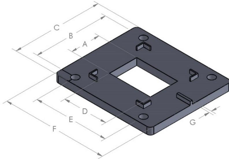
*Figure 9: EOS recommended calibration artifact created during "fine-tuning" build. Measurements collected from the artifact are used to generate beam offset, X scaling, and Y scaling values.*
