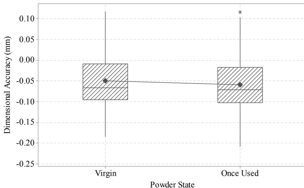
Figure 5: Box and whisker plot comparing dimensional accuracy between virgin and reused powder. Statistical testing indicated no difference between the two population means.
