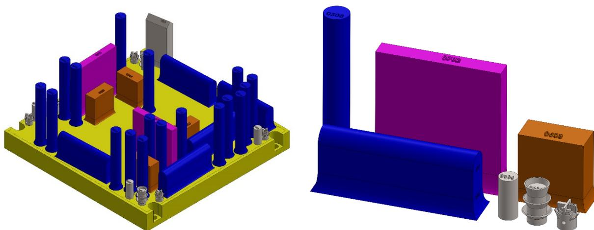
*Figure 1: Part layout on AM build (left). Both mechanical test specimens and witness coupons measured for dimensional analysis (right).*
