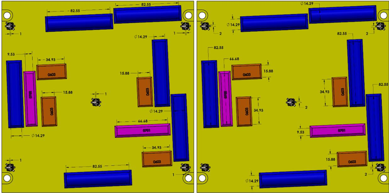
Figure 10: Nominal part sizes shown in the X measurement direction (left) and Y measurement direction (right).
