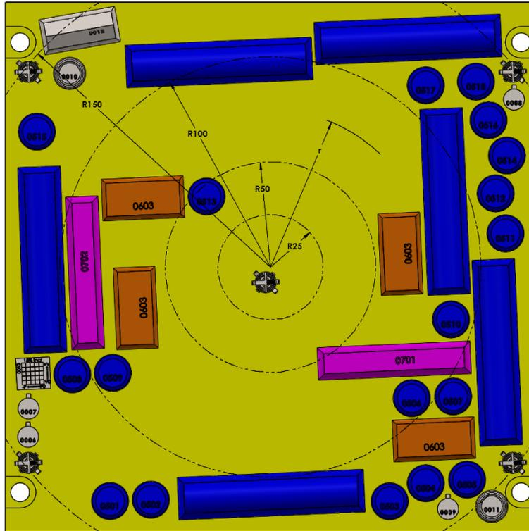
Figure 7: Illustration of various distances from the center of substrate. Dimensional accuracy measurements were analyzed according to the distance from the center of the substrate to the centroid of the part under measurement.
