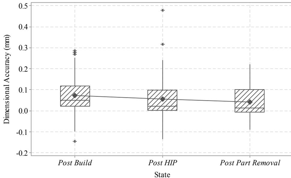
Figure 6: Box and whisker plot comparing the dimensional accuracy across three key manufacturing processes.
