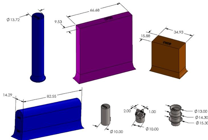
Figure 2: Nominal part sizes (diameters, lengths, and widths) of mechanical test specimens and witness coupons.
