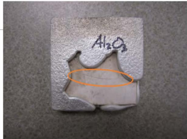
(b)  $\text{Al}_2\text{O}_3$  tile encapsulated in Al-Cu alloy exhibiting lack of complete encapsulation and tile cracking
