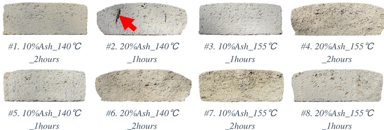
Figure 17 The cross section of sulfur concrete extrudate
