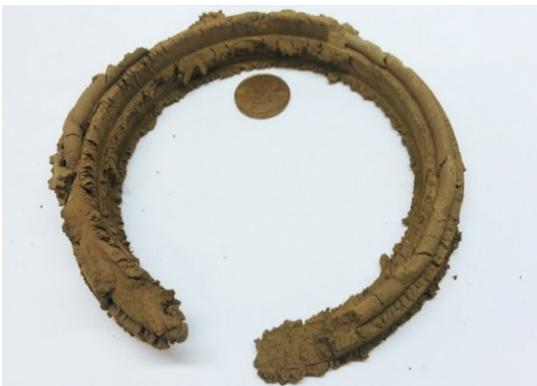
(a) Extruded sample with cracks on surface
