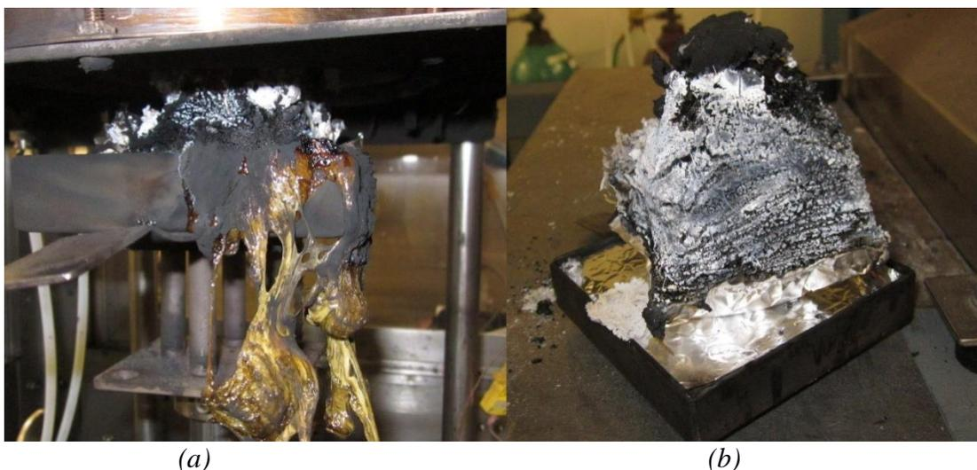
Figure 9: *ULTEM™ sheet ash from cone calorimeter test (a) AM sheet ash, with unburned material hardened from flowing over the side of the holder, and (b) Molded sheet ash, which was completely contained by the holder and foil wrapping.*
