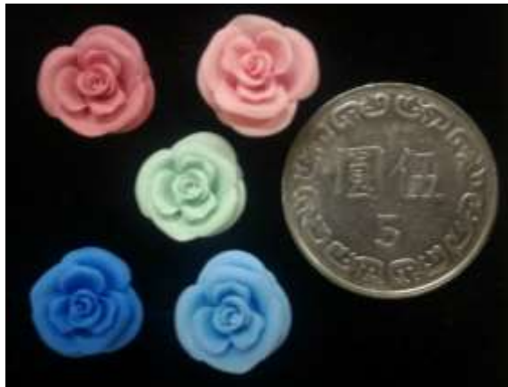
Figure 9: 3D printed Roses with Alumina using 3S process in different solid colors
