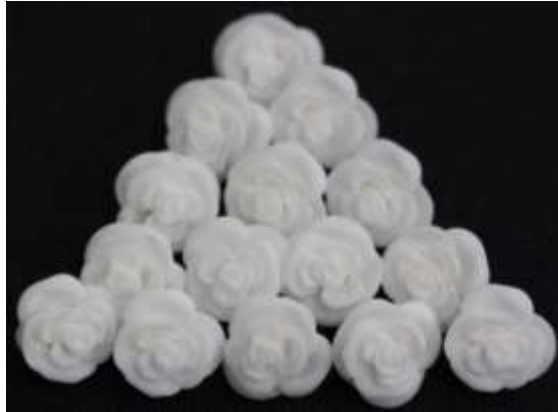
Figure 8: Resultant models of the roses after sintering
